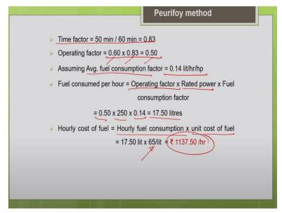
Now the time factor is directly given it is nothing but your working efficiency your machines working for 15 minutes per hour, 50 by 60 = 0.83 that is the working efficiency of your machine. Now the operating factor is nothing but time factor multiply by the load factor. Load factor is 0.6 time factor is 0.83 your operating factor is 0.5. Now you adjust your fuel consumption factor that is 0.14 liters per hour per horse power with the operating factor and the horse power of the engine.
