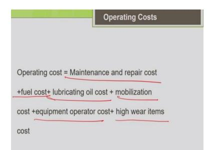
So what are all the components so far we have discussed under the operating cost let us summarize. So maintenance and repair cost your fuel cost, lubricating oil cost all these are consumables, the mobilization cost, equipment operator cost and cost of special items of high wear items. So all these things we have operating cost of the machine.
