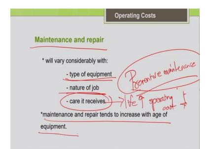
So now let us discuss about the operating cost one by one in detail the first one which we are going to discuss is about the maintenance and the repair cost. So this contributes to significant proportion of the operating cost of the machine. So basically as your machine age increases, as a machine ages obviously your repair cost will increased your repair and the maintenance cost is going to increase. Because the machine; has been subjected to more amount of wear and tear.
