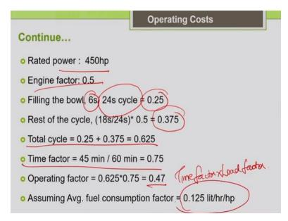
So the horse power of the machine is given the rated power 450 engine factor is given. So as I told you while filling the bowl it is consuming full power so it is taking 6 seconds out of the total production cycle time of 24 seconds to fill the bowl. During this cycle it is using full power, 0.25 into 1, so during the rest of the cycle that is 18 by 24 seconds it is using average power that is into 0.5.
