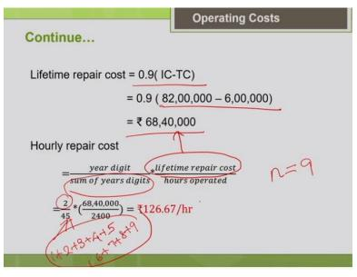
Now let us estimate the life time repair cost, it is nothing but it is given as 90 to 95% of the initial cost. So this value I am just checking it as the 90%, 0.9 into initial cost minus tire cost 0.9 into 82 lakhs – 6 Lakhs it is comes around 68,40,00 that is a life time repair cost. Now I can calculate the hourly repair cost for the they have asked you to find it for the second year of the equipment operation.
