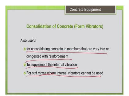
So, where do we use this form vibrators? Basically for thin sections as I told you where the internal vibration is not possible for a consolidating concrete in members that are very thin or congested with reinforcement where internal vibration is not possible. We go for form vibrators. And also in some cases to supplement the internal vibration in addition we can do the external vibration also.
