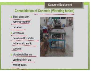
And the next one is the use of vibrating tables for consolidation. So, very commonly you could have seen this vibrating tables in the laboratories. So, in the concrete testing laboratories, you can see this vibrating tables. And it is also commonly seen in the factories like precast factories. So, you can see this vibrating tables. Basically these are steel tables with external vibrators mounted. So, the vibrators are mounted.
