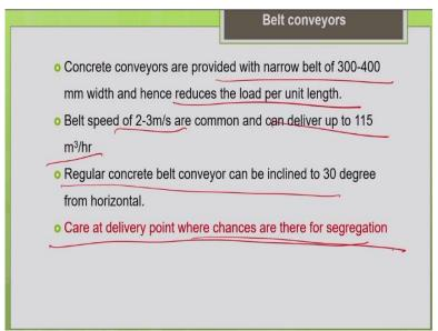
So, when compared to the belt conveyors which are used for the used for handling the other material. So, there are some differences in the belt conveyor which are used for conveying the concrete because a concrete is relatively denser material. So, generally we prefer to go for narrow belt. We restrict the belt width to say 400 mm. So, but commonly you can see a belt conveyor with width of up to even 1 meter.
