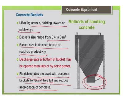
So, next is about the concrete buckets. So, very commonly we use this concrete buckets lifted by crane particularly for the high rise buildings. You can see that the cranes are used to lift the concrete buckets to the particular floor level to do the concreting work. So, not only the cranes, we can also make use of the hoisting towers or you can even use a cableway as I told you depending upon the job site location.
