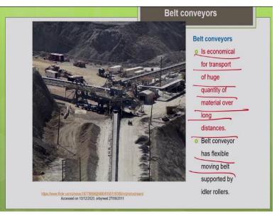
So, the next is about the belt conveyors. So, earlier belt conveyors were used only in the mining operations or tunneling operations. But nowadays, there are different ranges different configurations of belt conveyors. So, belt conveyors are very commonly used for material handling. We have portable belt conveyors, series conveyors. So, you can commonly see it in the RMC batching plant or asphalt batching plant or aggregate production plant.
