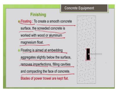
So, following screeding, the next stage is floating. So, always give some time interval between every stage of finishing and then do it. The main objective of floating is to create a smooth concrete surface. So, what you do is you either go for a wooden float like this or it may be even a metal one aluminum, magnesium, the metal floats are also available. So, with this metal float keep this blade flat and then smoothen the concrete surface.
