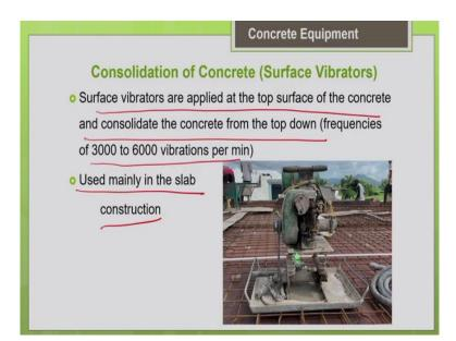
Now, let us move on to the surface vibrators. So, let us see how to do the consolidation of the concrete using surface vibrators. So, these vibrators as the name indicates the vibration is applied at the surface of the concrete and from the surface the vibration will be transferred throughout the entire depth of the concrete. So, generally speaking the internal vibrators are the best one.
