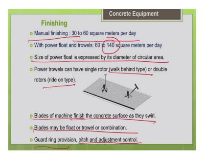
So, when you compare the productivity of the manual finishing with simple tools, you can see that manual finishing maximum productivity the finishing productivity is 60 square meters per day. It ranges from 30 to 60 square meters per day. But with a power float and trowels, you can go even up to 140 square meters per day. So, you can say that you can have a very high productivity using the power trowels and power floats.
