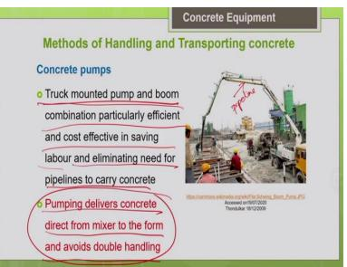
So, in some places the job site will be very much congested that it will not be possible to place the pipelines on the ground. So, in that case, you can go for this truck mounted pump and boom. Truck mounted, this is called as truck mounted pump and boom combination. So, your pump and the boom is mounted on the truck. This is your boom. Just like the boom of your crane. So, this is a boom.
