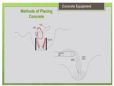
So, these are the schematic pictures which shows the right method of placing the concrete. Say for example, if you want to place a concrete into a concrete column formwork. So, we are going to do the concreting of column. So, you are going to deliver the concrete into this column
