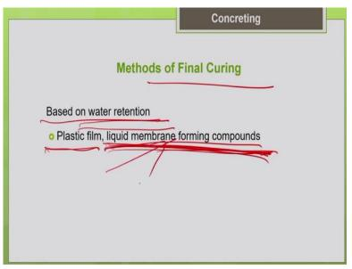
So, the other method which I told you is based on water retention. So, here what we do is we do not apply water for curing but we prevent the loss of water. So, how to prevent the loss of water? You cover the concrete surface with a plastic film or any polyethylene film and prevent the loss of water from within to outside environment. This is very commonly followed in places where sufficient water is not available for curing where there is water scarcity.
