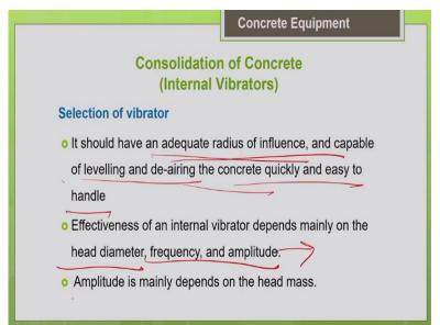
So, whatever vibrator you choose, it should have a adequate radius of influence so that you can have your desired consolidation rate. You can see your rate of concrete placement also varies. For a smaller vibrator, you can see 1 to 4 meter cube per hour. But for a bigger diameter vibrator you can have 19 to 38 meter cube per hour the concrete placement. So, depending upon the productivity needed, so, you have to make the choice of your vibrator.
