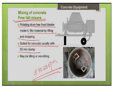
The first is about the free fall mixer. So, the conventional drum mixes what you see in your job site very commonly, is based on free fall mechanism. As the name indicates, the concrete here, we are going to discuss based on free fall mechanism of the material that means I can see the inside
