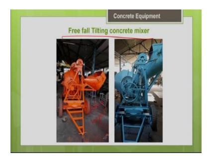
So, basically in this free fall tilting type of the concrete mixers, you can see this kind of wheel arrangement, you can see. So, with this wheel arrangement, you can change the angle of inclination of the drum. So, you can change the angle of inclination of the drum with this wheel arrangement. So, that helps you to tilt the drum.
