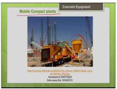
So, we have different configurations of the batching plant. You can also have a small batching plant, mobile compact plant, depending upon your requirement. You can see a small the cement silo, aggregate storage bins and the mixer machine. So, depending upon your job requirements, you can have a small batching plant also. So, as I told you, if your project site is very far away
