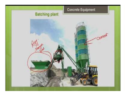
So, this is the real picture of the batching plant. You can see the aggregate storage bins. These are the aggregate storage bins. So, you have the belt conveyors to transfer. You have the mixer machine. You have the cement silos. So, the materials are conveyed by the belt conveyors to the mixer machine where the mixing is done.
