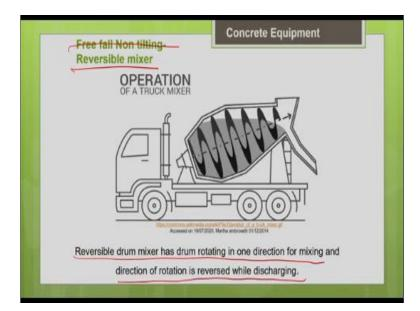
(Video Starts: 00:22:07) Your RMC transit mixer, it is also an example of free fall non-tilting reversible mixer. So, here also, you can see, there is only one opening. You have spiral blade arrangement inside. So, you have spiral blade arrangement inside. So, when you feed in the material, you have to rotate in one direction. So, when you want to discharge the concrete out, you have to rotate in the opposite direction.
