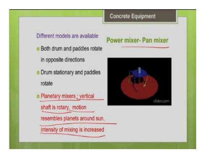
So, there are different configurations of the models available with respect to pan mixer. So, either the drum will be fixed, the paddles will be rotating or both the drums and the paddles will be rotating but in opposite direction. So, another popular model is planetary mixer. Why it is called as planetary mixer is, it resembles in motion planets around the sun, your paddles will be rotating about its axis.
