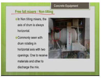
So, the next is about the free fall mixes non-tilting type. Here, I cannot change the angle of inclination of the drum. You can see that the excess of the drum is always horizontal. You cannot change the angle of inclination of the drum. Commonly, you can see this with 2 openings. So, one for feeding in the material and one for discharging the concrete out. So, this is a common configuration, you can see for a non-tilting type.
