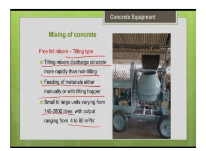
So, as I mentioned earlier, the tilting mixers discharge concrete more rapidly than non-tilting. So, particularly for the concrete, the time is very critical. Once you prepare the concrete, once you add the order to the cement, what happens is, cement will start the setting that is why as early as possible, they should just place a concrete in the desired position. So, that is very important with respect to the concrete.
