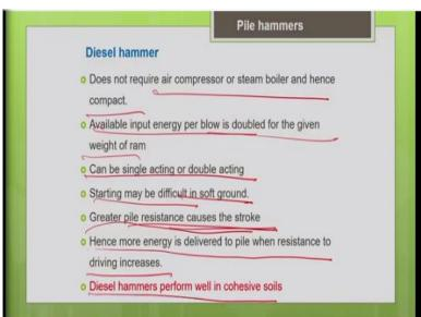
The main advantage is it does not require a separate air compressor or steam boiler and hence very compact. And the available input energy per blow is doubled for the given weight of ram, how it is double? Because of the explosive energy we get additional energy for driving, so it can be also either single acting or double acting. So, as I told you in a soft ground, the initiation of the process is difficult.
