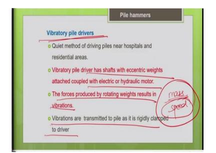
So, the last type of pile which we are going to discuss is about the vibratory pile driver. So, for whatever we discuss on impact hammers, which results in lot of noise production as we discussed earlier. And this method may not be feasible, if you are going to do a pile driving operation in a residential colony or near schools or hospitals where we need silent pile driving method.
