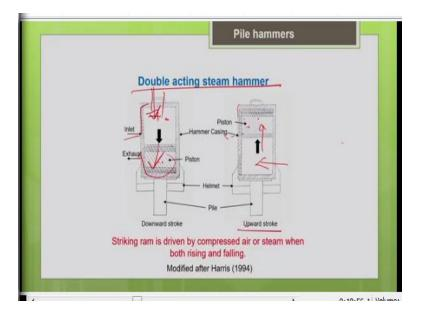
So, basically what to do here is, so this is a setup of the double acting steam hammer, you can see two cylinders one is the upper cylinder, other one is a lowest cylinder. Now in the upward stroke what you do is, you supply air into the lower cylinder. So, when you supply into this, this is a lowest cylinder, when you supply air into the lower cylinder, the hammer which was earlier in the lower cylinder will be pushed up into the upper cylinder.
