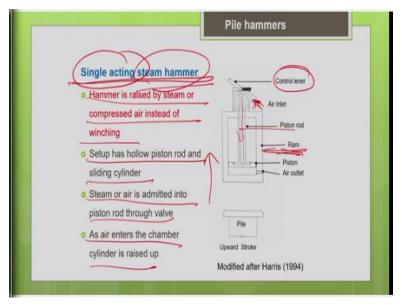
Next is your single acting steam hammer, so this is an improvement over the drop hammer. As a name indicates steam hammer, so it means you are going to use a steam energy, you can either go for steam energy or you can go for compressed air also. So accordingly, you may need a steam boiler or air compressor for this method. So, the name says single acting, that means you are going to use the steam energy only in the upward stroke.
