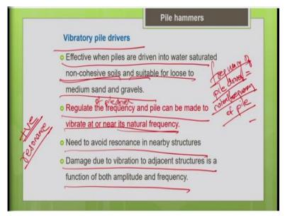
You regulate the frequency and the pile can be made to vibrate at or near it is natural frequency, you regulate the frequency of the pile driver and the pile can be made to vibrate at or near it is natural frequency. So, this will result in positive impact of resonance, which will make your pile driving operation easier. Another important thing is you need to avoid the resonance in the nearby structures, make sure that the frequency of the structure should not coincide with your pile driving.
