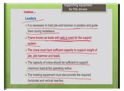
So, as I told you it needs some supporting frame structure to hold everything in position, so that you can maintain the proper alignment of the pile, so for that you need help of the needles. So, it is necessary to hold the pile and the hammer in position and guide them during installation. So, for that we need the frame known as lead, it has a rail, you can see it has the rail kind of arrangement, it is used as a support system for the pile driving operation.
