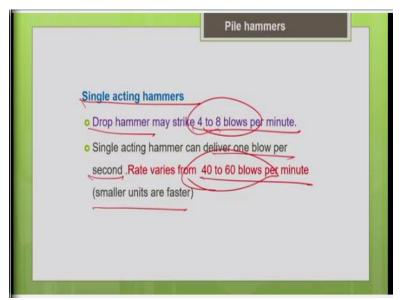
So, when you compare the productivity of your single acting hammer with the drop hammer, say earlier we discuss the blow rate of the drop hammer is 4 to 8 blows per minute. But your single acting hammer has a better productivity, it can go of a 1 blow per second. That means the blow rate is almost 40 to 60 blows per minute, even the smaller will more faster, when compared to the larger units.
