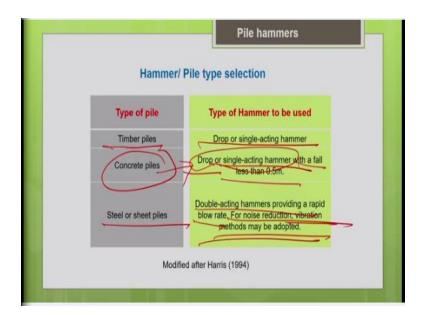
So, we have discussed about the functioning of different types of hammers and let us discuss about how to make the hammer selection. Your pile material type, the soil type everything is going to govern your selection of your pile hammer. So, with respect to material type as I told you particularly for the concrete piles you should be very careful, we should go for heavier hammer, heavier in the sense you can go for drop or single acting hammers which are basically heavier.
