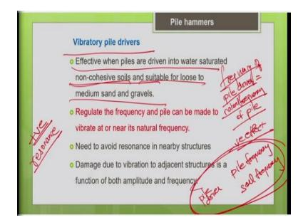
So, for what type of soil this is more preferable, this is more preferable for non-cohesive soil because that will respond easily to the vibration when compared to cohesive soil. So, this is particularly for water saturated soil, this is the right choice. So, this is effective in the piles are driven into water saturated non-cohesive soil and suitable for loose to medium sand and gravel because these kinds of soil will respond well to the vibration.
