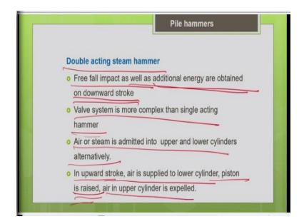
So, we have discussed about the single acting hammer, now let us move onto double acting steam hammer. As the name indicates double acting, so you are going to use the steam energy for both the upward stroke as well as for the downward stroke. So, that means you are going to use the steam energy for rising of the hammer as well as for the falling of the hammer. So, the freefall impact as well as additional energy or obtained on the downward stroke.
