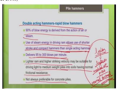
So, another important thing we need to know with respect to double acting hammer is in this most of the blow energy is the derived from the steam energy. Both for the upward stroke as well as for the downward stroke, the blow energy is derived mainly from the steam energy. So, 90% of the blow energy is derived from the action of air or the steam. So, that is why, for the double acting hammer we need not for a heavier hammer.
