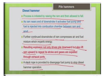
So, let me summarize the operation of the diesel hammer, this process is initiated by raising the ram and then it is allowed to fall. You have to raise the ram with help of any lifting mechanism the crane. As the ram nears the end of the downward stroke it activates a fuel pump, and the fuel is injected into the combustion chamber between the ram and the anvil. So, further continued downward stroke of the ram compresses the air and the fuel mixture, so that will impact the energy.
