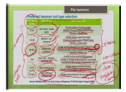
Now how to make the pile hammer selection with respect to your soil type, as I told you we can classify the soil into different categories. So, based upon there are some standard tests to categorize the soil into different categories. Like once this test is your standard penetration test where you find what is the number of blows needed for the standard penetration. So, based upon the number of blows you classify the soils into different categories are shown here.
