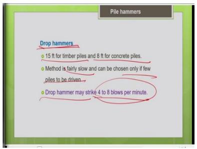
So, that is why for concrete piles the limitation of height of fall is given for the drop hammer as 8 feet, for timber pile it is 15 feet. And one more important thing to be noted is, this drop hammer method is very slow, it is fairly slow. So, if you have to drive only few piles, if you do not have a
