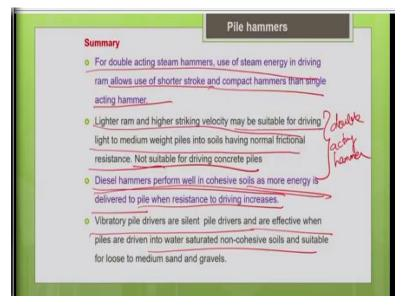
For double acting hammer, use of steam energy in driving ram allows use of shorter stroke and compact hammers than the single acting hammer. So, double acting hammers are basically smaller in size and they go with shorter stroke when compared to single acting hammer. So, they have basically recommended for the soil with normal friction resistance and for light to medium weight piles.
