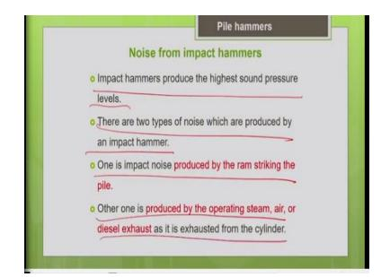
So, whatever hammers we discussed so far, a drop hammer, single acting hammer, all these impact hammers are noisy hammers, that means it results in lot of noise prediction during the driving operation. So, the impact hammers produce the highest sound pressure levels. So, there are different types of noises. One is because of the hammer the ramming against a pile head, that results in one type of noise.
