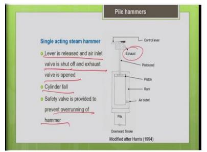
Now let us see how the downward stroke is done. Now what you do is you control the lever in such a way that the air inlet is shut off, you close the air inlet and all the air from the cylinder will be expelled out of the exhaust valve, so all the air now comes out of the exhaust. As the air is released out of the chamber, the hammer will fall down, so hammer falls down, so that is a downward stroke.
