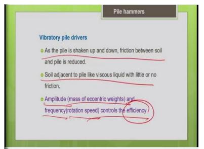
So, as your pile is shaken up and down, consider the friction between the soil and the pile will be reduced, so that will facilitate easy penetration of a pile into the ground. Because of the vibration, the soil adjacent to the pile will behave like a liquid, with little or no friction which facilitates penetration of the pile into the ground. Your amplitude of the vibration will depend upon your mass of the weights, eccentric weights inside your vibrator.
