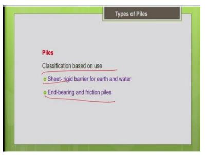
So, based on the application, so commonly, there are different types of uses of piles. So, I am just going to discuss few common applications, so one is a sheet pile and other one is your end bearing pile and friction pile.
