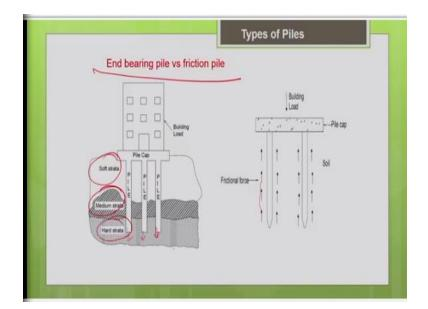
So, other types of applications are end bearing file and the friction pile, based on the mode of load transfer. So, particularly for the soil with poor bearing capacity and we go for this end bearing pile. So, the end bearing pile has to transfer the load through the weakest strata till it reaches it hard bearing strata which can carry the load. And the load is transferred through the end that is why it is called as the end bearing pile.
