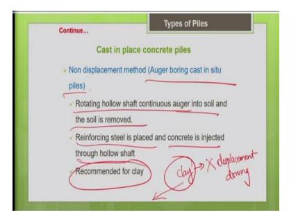
So, let me summarize, first you need to rotate the hollow shaft continuous auger into the soil is the rotary method as I told you. So, you have the rotating hollow shaft continuous auger. So, it has a spiral or helical auger as I showed you, which can easily bore the hole into the ground and it can remove the soil out of the hole. So, the soil is removed and the reinforcing steel is placed and the concrete is injected with the help of a tremie pipe.
