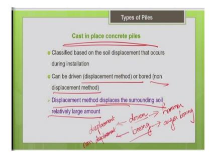
So, what is this cast in situ concrete piles, what are the methods of making cast in situ concrete piles? Here also based on the process of installation, you can classify it further into displacement method and non-displacement method. See, when you do the installation process, say if your installation process is going to disturb the surrounding soil to a greater extent, say if it is going to displace the surrounding soil to the greater extent, then it is called as displacement method.
