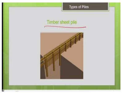
This is the picture of the timber sheet pile, as you know that timber is the oldest material. So, oldest building material we have been using this material for so many centuries, even now we use it wherever the timber is abundant.
