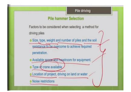
So, now let us see what are all the basic factors which governs the pile hammer selection. So, obviously we have to select the pile hammer depending upon the type of a pile. So, what will be the size of a pile, weight of a pile according to that you have to choose a weight of the hammer. So, the common guideline is your weight of the hammer should be at least equal to the weight of a pile that is a common guideline, ideal case.
