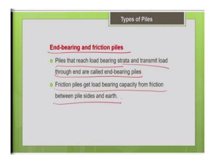
So, this is what we discussed just now. Piles that reached a load bearing strata and transmit the load through the end are called the end bearing piles. Friction piles get the load bearing capacity from the friction between the pile sides and the earth.
