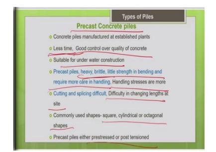
So, far we have discussed about the cast in situ concrete piles. So, there are two ways you can go for the displacement method there is the driving method or you can go for the non-displacement that is boring method, and we have discussed about the auger boring. So, now we are going to discuss about the precast concrete piles. So, they are going to be made in the factory in control condition.
