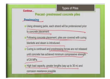
Because as I told you concrete piles, say for example, the precast concrete piles, it is a normal conventional reinforced concrete pile. If the length is say, now commonly we do not go beyond 15 meters. But if you go for pre-stressing method, we can even go up to 30 meters because you can easily resist the handling stresses, so that is one advantage of pre-stressing. So, let me summarize what we discussed earlier in the previous slide.
