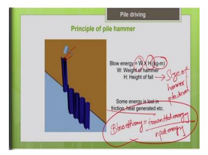
First let me introduce to you what is the basic principle of pile driving. So, it is just like how you drive a nail into a wall with a hammer, the same way you are going to drive a pile into the ground with a hammer. So, you are going to blow the hammer on the top of the pile, so what is the blow energy? So, it is going to depend upon your weight of the hammer and the height of the fall of the hammer, so that is what is going to give you a blow energy in Kg meter.
