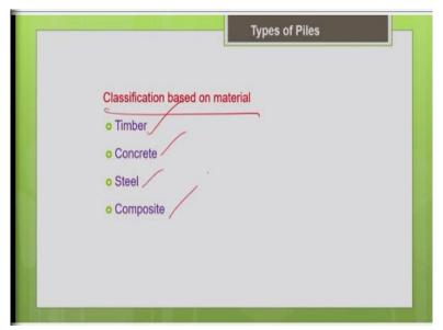
Now we have discussed the few types of piles based on the application or the use. Now let us see the classification based on the material type. So, we can classify it into timber, concrete steel and composite piles.
