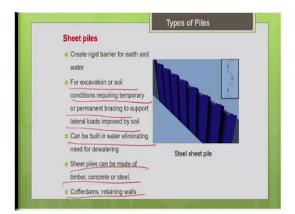
First let us see what are these sheet piles? The sheet piles so we might have seen this kind of steel sheet piles, so they are with interlocking joints, you can see that. So, they act like a rigid barrier for earth and water particularly during excavations or trenching. So, to protect the trench from the collapse, to prevent the trench from the collapse of soil, we go for this kind of sheet piles.
