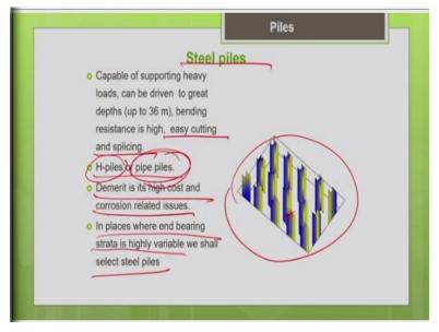
So, with this let us move on to the steel piles under the concrete piles we are discussed about cast in situ as well as precast concrete piles. So, now let us discuss about steel piles, the main advantage of steel piles is, it is load bearing capacity is significantly high when compared to concrete piles. Particularly it is a unit load bearing capacity, it is going to be very high.
