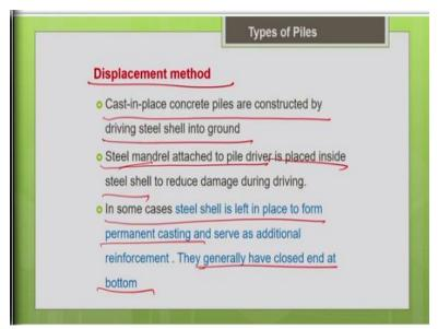
So, let me summarize what we discussed earlier on the displacement method. So, cast in place concrete piles are constructed by driving the steel shell into the ground, shell is your casing and the steel mandrel is attached to the pile driver is placed inside the steel shell. So, why the mandrel
