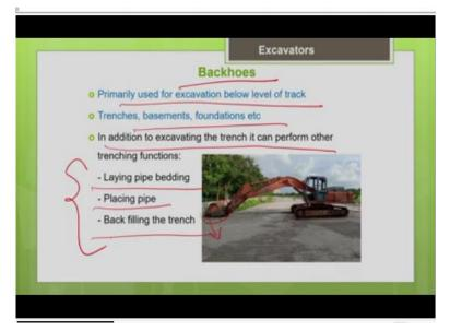
So, now let us discuss about the backhoes. So, you can see that the basic parts and operation are similar for both the machines but only thing to be noted is the digging motion of the bucket is in downward direction. So, it is preferred for the deep digging below the ground level, this machine is used for the digging below the ground level. So, mainly used for excavation below the level of track.
