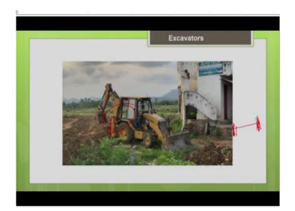
So, this is the combination of front end loader and backhoe. In some places you may need this combination because I may have to use a backhoe for excavating below the ground level, at the same time I may need a help of a front end loader to transport the material to a dumping position, when both are needed together then you have to go for this front end loader backhoe combination.
