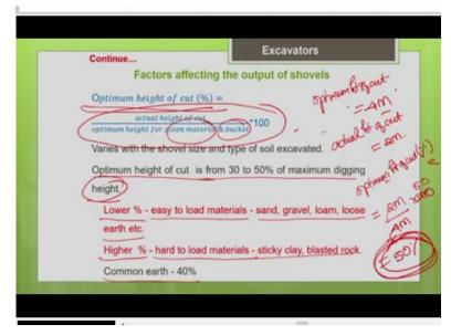
Now, let us see how to know the optimum height of cut for the machine. So, optimum height of cut require for a particular machine depends upon the dimension of the machine as I told you. So, this will be equal to based on studies they found that it is equal to 30 to 50% of maximum cutting height obviously, you know that for every machine for every shovel, I can get the information on what is the maximum cutting height from the manufacturer, what is the maximum cutting height.
