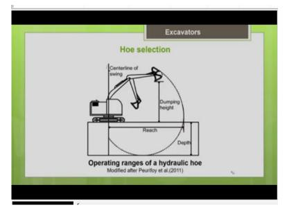
As we discussed earlier for the front shovel here also, these are the important parameters which helps you in the selection, what is the maximum dumping height possibly with the machine? What is the maximum digging reach possible with the machine when you completely extend your arms, when it completely extends it you can get the maximum digging reach possible that will give you the working radius possible.
