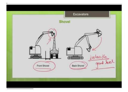
So, basically, shovels can be divided into 2 types based upon the digging motion of the bucket. So, in the first picture, you can see that the digging motion of the bucket is in upward direction. So, it is an upward direction. So, that means the bucket is moving away from the machine. So, that is called as a front shovel, in backhoe or the back shovel, you can see that the digging motion of the bucket is a downward direction.
