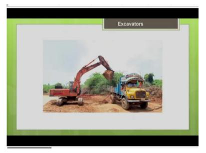
So, this video again shows you how the truck is commonly placed very close to the backhoe. (Video Starts: 50:58) (Video Ends: 51:39) As I told you, the angle of swing will be 90 degree, the horizontal angle should be 90 degree between the loading and the dumping position. So, the truck should come very close. So, that backhoe will be able to excavate the material and load it into the truck.
