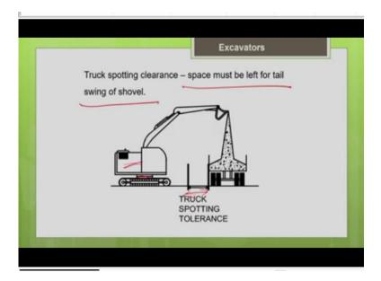
Another thing to be noted is truck spotting clearance. That means, as I told you, it is preferable to place a truck closer to the excavator. But at the same time, note that there should be some space left for the tail swing of the shovel. That means now you can have a complete 360 degree swing, you have a slewing ring here, you can have a complete 360 degree rotation about the mounting.
