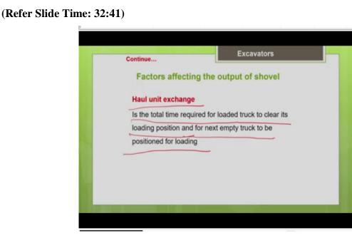
Other important factor is haul unit exchange time. That means the time needed for the loaded truck to leave its position. And for a new truck that is an empty truck to take the position. That
