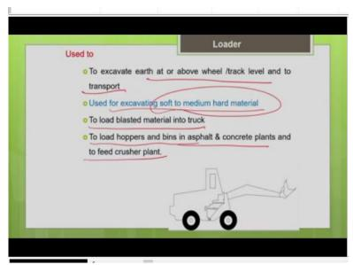
So, let me just summarize. So, basically the loader is good in excavating at or above the wheel or track level and also it is used to transport the material to certain economic haul distance. We have discussed the haul distance, it varies depending upon the mounting of the machine and it is designed for excavating soft medium hard material, with softer medium hard material, you can get a good productivity.
