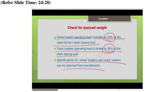
And we have to check whether the operating load of your machine that is the load in the bucket should be well within the full turn static tipping load prescribed by the manufacturer for that particular machine. So, the load in the bucket should be well within that. So, we should go for a very high factor of safety. The factor of safety depends upon the mounting of the machine.
