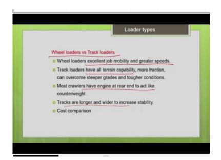
So, first let us compare the wheel loader versus the track loader. Obviously, as you know, wheel loader will give you high mobility. So, wherever you need higher speed and greater haul distance, you can go for the wheel loader, with wheel loader I can go for economical haul distance of up to 200 meter. So, excellent job mobility and greater speed, but the main advantage of track loader is it has all terrain capability.
