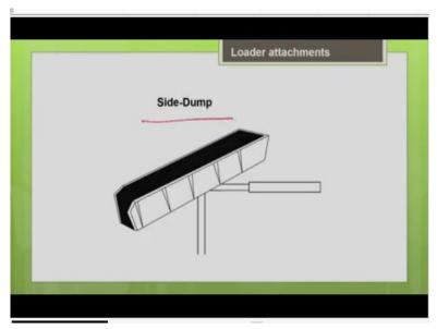
This is the side dump attachment. This is a schematic picture of the side dump attachment, which you can use it in confined areas where you want to do the dumping on one side, I do not want to do the dumping in the front end, but I wanted to do the dumping either to the left side or to the right side, then I can go for this kind of side dump attachment.
