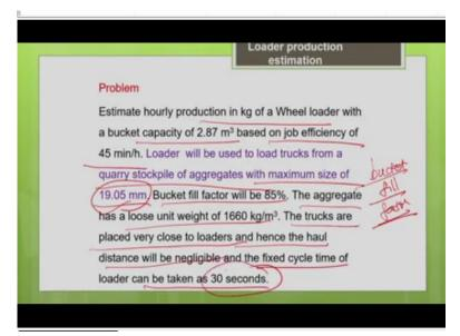
Now, let us work out the problem and see how to estimate the productivity of the loader. So, estimate the hourly production in kg of a wheel loader with a bucket capacity of 2.87 meter cube, the rated bucket capacity is given 2.87 meter cube, it is a wheel mounted loader, job
