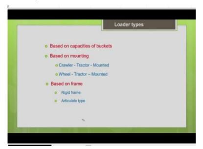
Now let us see what are all the types of loaders you can classify the loader based upon the capacity of the bucket or based upon the mounting or based upon the frame. So, based upon the capacity of bucket, you have a huge range of the capacity say starting from less than 1 meter cube say 0.2 meter cube to as big as say 15 meter cube bucket is also available. So, depending upon your requirement you can go for the corresponding bucket the size accordingly.
