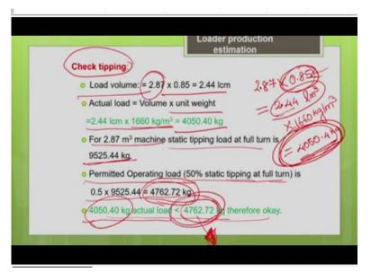
Now, let us work out a solution, the first step will be you have to do the checking for tipping. So, particularly for the front end loader as there are more chances for the machine to tip forward if you are going to overload the bucket. So, that is why we have to check for tipping. So, we have to make sure that the weight of the load in the bucket is going to be well within the full turn static tipping load defined by the manufacturer.
