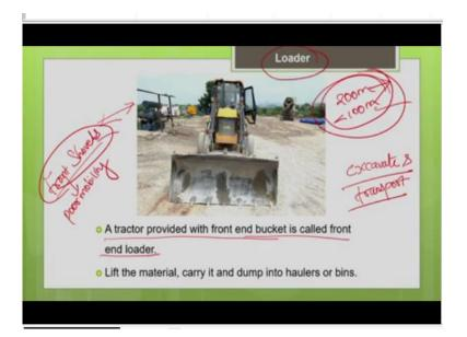
So, as the name indicates, the front end loader means it is basically a tractor with a bucket at the front end a tractor provided with the front end bucket is called the front end loader. So, you might have seen this front end loader very commonly in many project sites. So, the basic difference between this machine and the; earlier machines which have discussed like bulldozer and scrapers is that.
