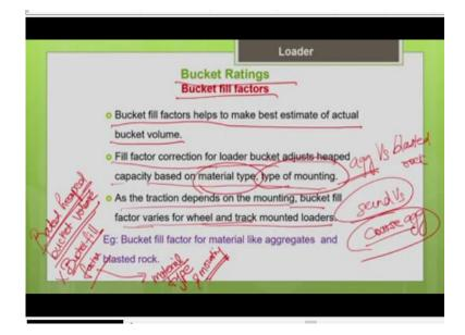
Now, let us see about the bucket ratings, see the manufacturer provide you the information on what is the heaped capacity of the bucket. So, this bucket rating is done by the manufacturer in a standard manner with a particular material, say they heap the material at a standard angle of repose say is 2 to 1 and then rate the bucket based on that. So, that bucket rating, we are going to use it for the estimation of the productivity of the loader.
