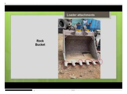
This is a picture of the rock bucket which shows the V shape cutting edge, you can see the V shaped cutting edge with this, even these bucket teeth is bolted on you can easily replace the bucket teeth when it gets worn out. So, this is particularly use for handling the rocks. When you are working with the loader in the quarries to handle the blasted rock or a short rock, then you have to go for this rock bucket, which can easily loosen the rock and load bucket.
