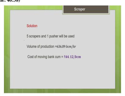
The solution is we are going for 5 scrapers and 1 pusher. The associated production value is 636.89 bank cubic meter per hour and the unit production cost associated is rupees 44.12 per bank cubic meter. So, this is how we have to estimate the productivity and the unit production costs for the
