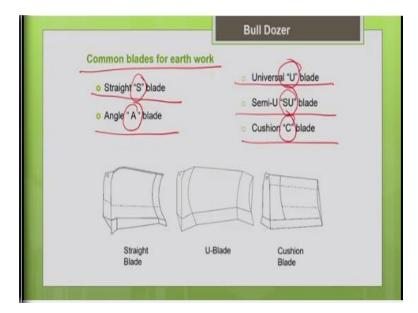
Now let us look into what are all the different types of the blade. These are the common blades which are used for the earthmoving operation, straight blade, angle blade, universal U blade, semi U blade and cushion blade. So, these are the standard notations used S refers to straight blade, A for angled blade, U for universal, SU for semi U and C for cushion blade. So, we are going to discuss all these blades one by one in the upcoming slides.
