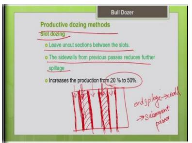
So, one such method is your slot dozing method, slot dozing. So, basically how to carry out this slot dozing? You have to divide your land, your area where you are going to do the dozing operation into many parallel cuts divided into parallel cuts. So, if you have a larger area, it is easy to implement this method. Divide your area into parallel cuts and allow the bulldozer to move through alternative cuts first, let it move through alternative cuts first.
