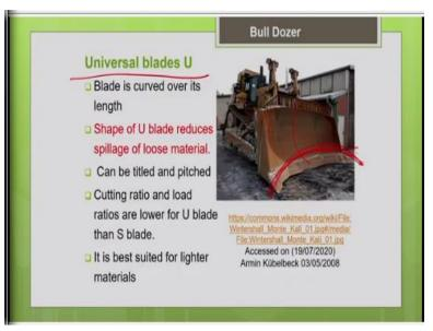
Universal blade, U blade, this is what I mentioned little bit earlier, like this blade has a curvature in the horizontal plane also. All the blades have the curvature in the vertical plane; in addition, these blades also have the curvature of the horizontal plane.
