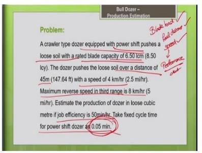
So, you know the blade capacity, you know the blade load, that is known. So, you know the haul distance the dozing distance is known, so it is known, you know the speed of the machine. If the speed is not given in that case you have to go for the performance chart, with the help of performance chart you have to find the speed. But in this problem speed is given to you directly. **(Refer Slide Time: 1:41:05)**
