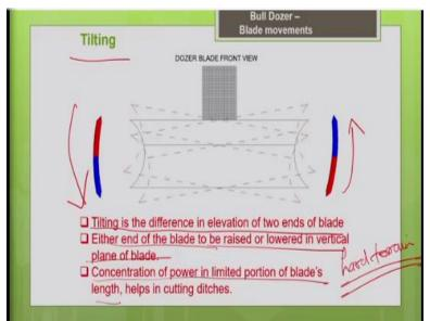
Now coming to tilting, tilting is the next type of movement. So, basically this is a movement in the vertical plane. So, you can raise one end of the blade and lower the other end. So, tilting is a difference in the elevation of the 2 ends of the blades; it is a movement in the vertical plane, why should we tilt the blade?
