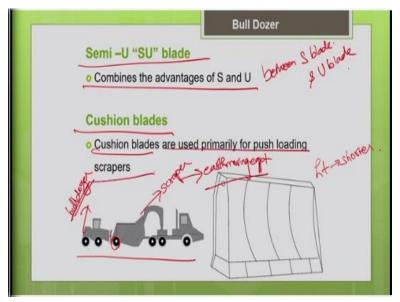
Now let us see what is this SU, semi U blade. It is something between straight blade and U blade, it is between S blade and U blade. That means it is dimensions bigger than the S blade but smaller than the U blade. Similarly cutting ratio is the lesser than the S blade but better than the U blade. So, it is something between the S and U blade. So, accordingly you have to make the choice according to your requirement.
