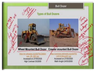
So, what happens if you go for say when you consider your track mounted or crawler mounted bulldozer. Here the coefficient of traction says it may be approximately 0.9 on a clayey terrain. So, here for the wheel mounted the coefficient of traction maybe only say 0.5. So, for the same weight of the machine since the coefficient of traction is very high obviously you can see with the usable
