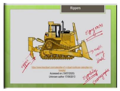
So, other application you can see it can be used as a ripper. So, for this tractor you can see a front end you have this blade earthmoving blade, this is the earthmoving blade, so at the rear end, you have this ripper. So, this is similar to plough what we use in farming. So, basically when we discuss about the earthmoving operations, the steps involved in the moving operations, I told you like the first step is we should loosen the earth before digging it.
