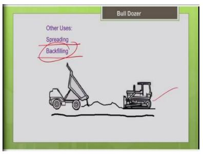
So, what are the other uses? The bulldozer can be used for spreading, backfilling. So, here you can see the example of spreading your truck. Very commonly you can see this in a road construction, the hauling equipment that is a truck, so it will dump the material and your bulldozer is used for uniformly spreading it and it will compact it to the regular thickness, so it helps in spreading the material.
