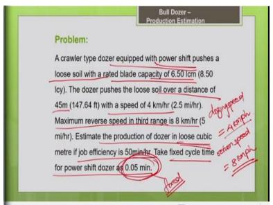
Now let us workout another problem a different approach of estimation of the productivity. So, in this a crawler type bulldozer is given, this equipped with power shift mode. So, automatic gear change, it pushes a loose soil with blade capacity 6.5 loose cubic meter. So, the blade capacity is given to you 6.5 loose cubic meter, and the dozer pushes the loose soil over a distance of 45 meters.
