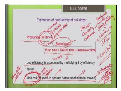
So, for that you need to know unit cost is nothing but cost per loose meter cube. Say I am going to find it in the loosen state cost per meter cube of earth moved, I need to calculate. It is nothing but your hourly cost associated with the machine divided by the hourly productivity. If we know these 2 data I can calculate. So, by now you should be knowing how to estimate the cost associated with the machine.
