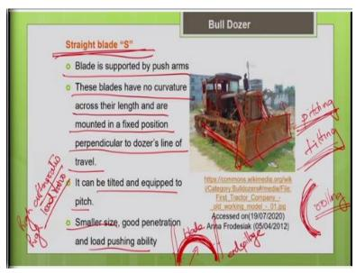
So, first we are going to discuss about this straight blade. Straight blade it is denoted as S, S blade. As the name indicates straight that means your blade is fixed straight perpendicular to the direction of the travel. So, this blade I cannot either angle it to left or right angle it to right, angling is not possible with this blade. It is fixed perpendicular to the direction of the travel, so that we have to note it.
