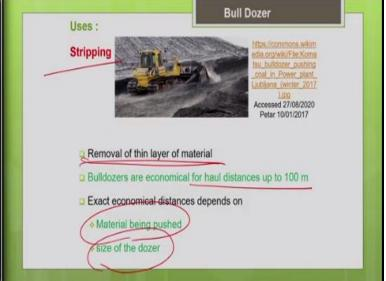
Then stripping, stripping is a very common operation in the construction project site. So, you know that stripping is nothing but removal of the top layer of the soil. So, if the top layer of the soil is weaker one with lot of vegetation, so you have to remove the top layer of the soil. So, depending upon a depth to which the vegetation is available in your soil accordingly you have to remove the top layer, so that is what is stripping.
