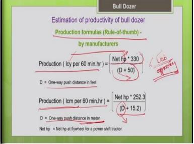
So, there are some thumb rules available provided with a equipment manufacturers. So, if you know the horsepower of the tractor and if you know the dozing distance, one-way push distance you can directly estimate the productivity of the bulldozer, these are thumb rules. It is nothing but your say net horsepower multiplied by 330 divided by D + 50, D is your one-way push distance or dozing distance in feet.
