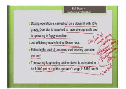
Then other things like operator the curve was drawn for excellent operator skill. So, in our problem the operator skill is average. So, accordingly you have to choose the correction factor and apply. So, your correction factor is going to be less than 1, because it is average is going to reduce your productivity. Similarly, the material type, material type is non-cohesive silty sand, so that will definitely reduce the productivity.
