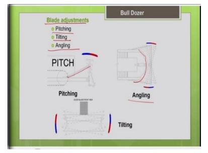
So, what are all the possible blade movements with the bulldozer blade? As I mentioned earlier, the movements which are possible depends upon the connection between the tractor and the bulldozer blade. In some bulldozers you can see this kind of C frame connection between the tractor and the blade. So, those tractors will facilitate certain kind of movements like angling.
