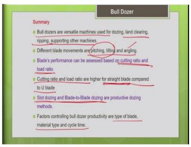
So, now we have come to the end of the lecture on bulldozer. So, let me summarize what we have discussed so far. So, as you know that bulldozers are versatile machines, so because it is used for different applications. So, not only for the earthmoving operations, we can also use it for cutting the trees, ripping the rocks and for assisting other machines. So, it is used for n number of applications, so that is why we called as a versatile machine.
