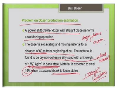
In this problem we are going to estimate the productivity of this power shift crawler dozer. So, power shift, so it is automatic gear change, so you can assume the maneuver time. The dozer is with a straight blade, it performs a slot dozing operation. The slot dozing operation you know that we adopt it, so that we can reduce the end spillage and you can increase the productivity of the bulldozer.
