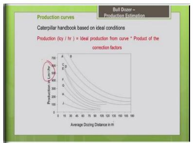
I hope you remember the sample of production curves which I have shown you earlier. So, if you know that dozing distance I can find the production curves. So, in this case the dozing distance is given as 60 meters. So, corresponding to your dozing distance if you know the model you can calculate the productivity. So, these curves are just some sample curves.
