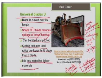
So, you can see the curvature in the horizontal plane in the form of U. So, what is the purpose of this U? So, that I can contain the material within the blade, so these are generally larger blades,
