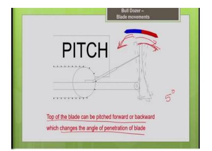
So, what is this pitching? Pitching means, the top of the blade is pitched forward or backward. That means you are moving the top end of the blade either forward or backward. So, this top end of the blade is moved forward or backward. So, why should we move it forward or backward? So, accordingly you can change your angle of cutting, accordingly you can change the depth of penetration of your blade.
