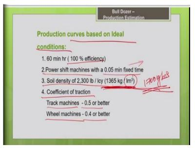
So, as I told you these production curves are drawn based upon ideal conditions. What are all ideal conditions? It is drawn assuming 100% job efficiency, that means your machine is going to work for 60 minutes in a hour, so that is what is the assumption. But in your real project site, your machine will be working just for 30 minutes or 45 minutes or 50 minutes. So, you have to apply the correction factor accordingly.
