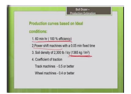
And hope you remember these curves are valid only for these ideal conditions. So, 60 minutes hour but in your project in this problem we found that the machine is working for 50 minutes an hour. So, you are supposed to apply the job efficiency, you have to apply the correction factor accordingly. So, this curve is applicable for power shift mode, automatic usage. So, in this problem also you have the automatic gear change, so no need to apply the correction factor.
