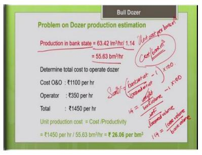
Now the next part, after estimating the productivity, now we are supposed to estimate the unit cost of production, unit cost stop earthmoving operation. So, how to do that, and they asked you to calculate unit cost per bank meter cube. So, that is what is asked in the problem cost per bank meter cube we have to calculate that. So, we need bank meter cube, but what we have calculated so far is your loosened volume.
