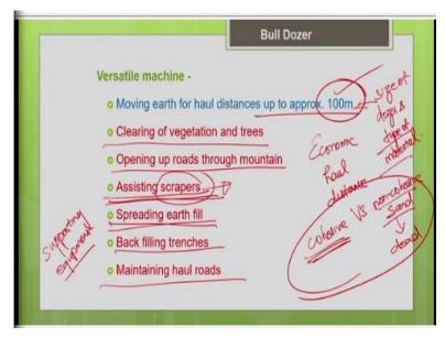
So, this bulldozer is basically a versatile machine. So, it can be used for different types of applications in a construction project site. So, before you select an earthmoving equipment for your particular activity or your particular job, you should know what is the haul distance actually
