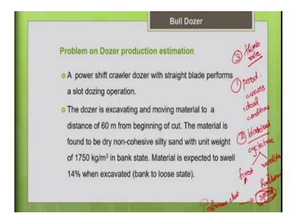
So, using production curves, which are drawn for the ideal conditions? So, we choose the value from the corresponding production curve which is supplied by the manufacturer. And apply the correction factors according to the project conditions and find the actual productivity for the project conditions, that is one way. The other method we learnt is, so we need to estimate the blade load, we need to know the blade capacity and then we need to determine the cycle time.
