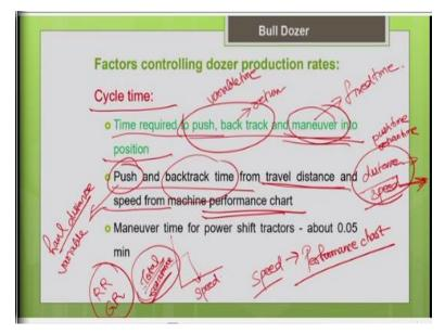
So, now let us see how to define the cycle and estimate the cycle time of the bulldozer. Say the bulldozer is used for earthmoving operation, how to define one production cycle of bulldozer? So, basically the bulldozer will cut the earth, once the blade is full, completely loaded, it will just push the earth till the dumping place, then it will return back to it is original position where you wanted to do the dozing operation again.
