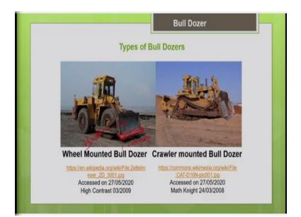
At the bottom of the blade, you can see a plate border. I mean this is the blade at the bottom what you have is the cutting edge; a steel plate is bolted to the bottom portion of the blade that is called as a cutting edge. So, generally this cutting edge gets worn out faster depending upon the usage, you may not replace the blade frequently, you need to replace only the cutting edge frequently.
