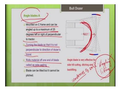
Now let us move on to the next type of blade that is the angle blade. So, these angle blades as I discussed earlier they are connected by C frame. The C frame is connecting the tractor and the blade. So, because of this C frame, it facilitates the angling moment. So, you can see the angle can be turned left or turn right to maximum of say 25 degrees. So, it is mounted on a C frame and can be angled up to a maximum of 25 degree left or right of the perpendicular of the tractor.
