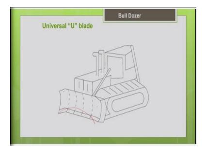
So, this is again a schematic sketch showing the U blade connected to the bulldozer, you can see they are larger in dimension and they have a U curvature. And you can see the wings attached on both the ends.
