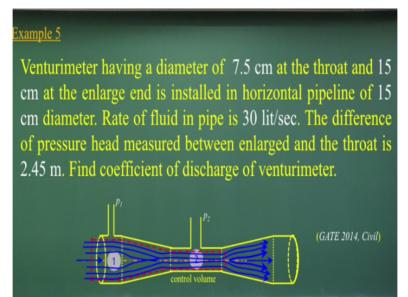
The example 5, which is a very simple problems on venturimeter as given in this figure.
