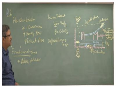
This is what the water jet and that what which strikes the deflector turns 45 degrees and if the velocity of jet leaving the deflector is 4 meter per second, the V jet is equal to 4 meter per second and the discharge the Q is equal to 0.1 meter cube per second. Then we have to find out what could be the force acting on the spring. This is what the problems.
