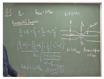
That there is a venturimeter with having the diameter of 15 centimeters is reduced to the 7.5 centimeters, which is installed on a horizontal pipeline. And the rate of the
