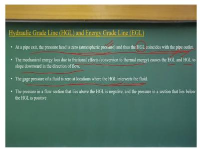
Now very basic things we should understand it, whenever a pipe exit, that means flow is going out. The pressure head becomes atmospheric pressure, no doubt about that. And that is the reason, the hydraulic gradient lines coincidence with the pipe outlet. So, when the pressure head becomes zero, that is what we said it, in case of open channel flow, when there is no pressure, is pressure is atmospheric pressure, that the surface becomes hydraulic gradient line.
