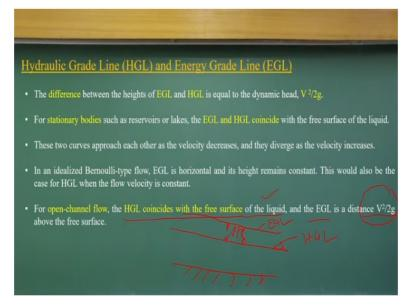
And okay, we are not discussing about open channel flow heads, but in case of open channel flow, the hydraulic gradient lines coincides with the free surface of the liquid okay. Because there is no pressure head. So, whatever the water surface free surface, that what will be hydraulic gradient line and the energy gradient lines will have a included the velocity head above the free surface. That means, if you consider a open channel flow, this is the free surface.
