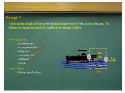
Let us have another examples very, interesting examples that a body is moving with a still waters of 6 meter per second produces water velocity 4 meter per second at 1 meter ahead. That means there is a distance between these two points is 1 meters, this is what 6 meter per second, the flow is, there is a reservoir type of conditions where the still waters are there and the velocity at this point is 4 meter per seconds.
