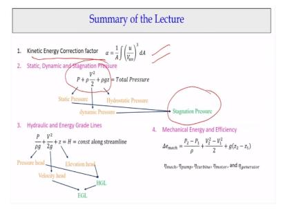
And that is the same things and this times we talk about the kinetic energy corrections factors, how we need to be compute when you have the velocity distributions is uniform. And we also seen Bernoulli equations, we can represent it in terms of the pressures, static pressures, dynamic pressures and hydrostatic pressures and two of the components that can represent us the stagnation pressures.
