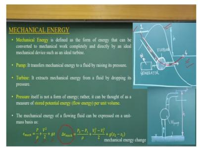
Now, let us consider is the problems when we generally use as a engineer having a pump and turbine systems. As you know it, the pump is transfer from mechanical energy to fluid by rising pressures, okay. Transfer the mechanical energy to a fluid. So, fluid gains the energy
