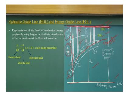
Now, another interesting applications of Bernoulli equations is that energy gradient line and the hydraulic gradient line. This is very great simplifications of the fluid flow problems. Like you may have fluid flow problems with pipe arrangement, the dock arrangement and all. Any flow, as I say that, it can have the flow distributions. But as total energy, along a streamline, if you can draw a streamlines and you want to quantify how these energies are changing it, okay,
