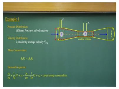
And we need to compute it in terms of average velocities. So, we are not considering is turbulent or laminar velocity things. We are not putting any kinetic energy correction factors, which supposed to be done it, but in this case we have not done it. We just apply the mass conservations and the Bernoulli equations assuming that there is a uniform flow distribution, it does not happen like that. We use the average velocity here.
