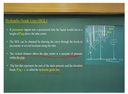
That is what I have explaining it that, so the basically piezometers and the hydraulic gradient line what I have said it and the hydraulic gradient line has some of the static pressures and the elevations. And the vertical distance above the pipe center is measure of the pressure within the pipe, okay. Within the pipe, what is the distance above the pipe centers, is a measure of the pipe pressure within this.
