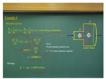
And then if I substitutes the Bernoulli equations, okay, along this constant lines. So basically if you look it, these two head, the pressure head and the z1 z2 is not given to us, but that is what will be reflect in terms of piezometric head. That is what is given the difference
