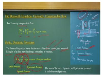
Now, let us come back to this Bernoulli equation what we have derived, that in case of unsteady compressible, will have the two integrals component. Then we have V square by 2 gz, which is the elevation head is equal to the constant. But in case we make it the steady and incompressible, then we get it these three forms as earlier I discuss it, this is summations of three energies, flow energy, which is because of the pressure at that locations.
