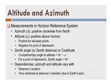
So, I am going to measure altitude and azimuth in horizon reference system. Remember, we are using the term reference system because it is just a concept now we are not realise
