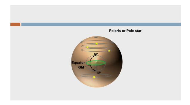
So, here I am showing you the earth well and there is a ellipsoid I am showing instead of earth. Let us assume that earth is a ellipsoid and so, I am showing you with the blue line which is vertical here, the line that is rotation axis of earth that is joining the North Pole and South Pole. Then we have a green circle which is equator and, then we have a dotted line which is showing the Greenwich meridian.
