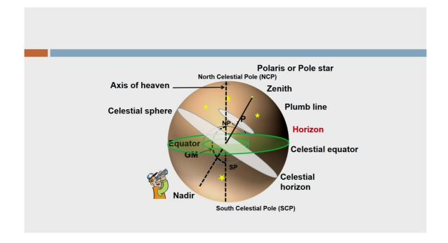
So, because we are calling all the stars has heavenly bodies or stars, right. So, same way, we are calling this axis which is passing through North Pole and South Pole of the earth or rather if I am extend the rotation axis of the earth. So, this axis is called axis of heaven.
