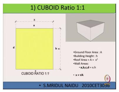
So somebody might take something like a cuboid, the ratio is 1 is to 1, ground floor area is A, building height is H let us say, so roof area is x square wall areas are x into H if it wall 1 is to 1. So x obviously one can find root x under root A.
