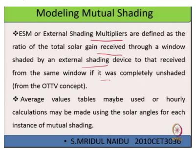
Then external shading multipliers they are essentially the ratio of the total solar gain received through the window shaded by an external shading device to that received from the same window if it was completely un-shading.
