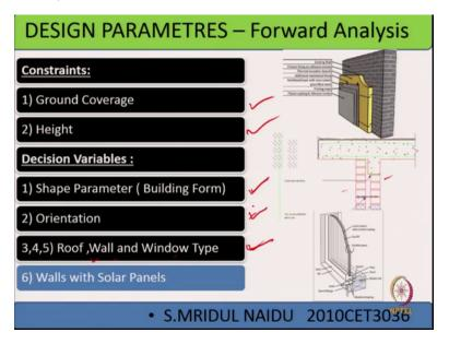
Now what are the factors which go into affects the energy efficient building design? First of all of course this ground coverage that will be part of the building itself, so that is the recommend functional recommend and that is my for my constraint in the sense that I have to ensure a particular level of ground coverage, height.
