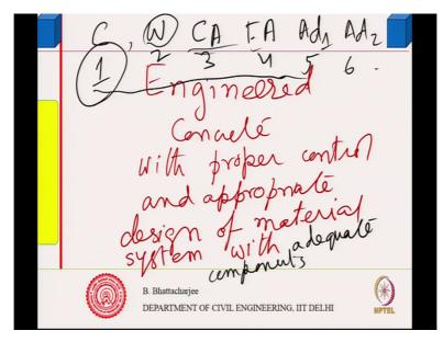
In other words I say that engineered concrete with proper control and appropriate design of material system with you know possibly not one you know normal concrete is essentially normal concrete is essentially cement that is one component, water the second component, say coarse aggregate third component, fine aggregate fourth component.
