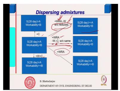
But supposing I am using admixtures like water reducing agent WRA then using this you know this WRA I have added I will reduce the water and then I can reduce the automatically keep the cement same. I need not increase the cement I can keep the cement same or I can design the system of course, I might even reduce the cement or you know accordingly I can do so what is just add WRA water will reduce W by C reduce therefore I get higher strength.
