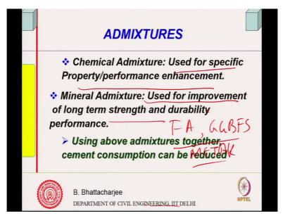
So it has to be engineered concrete and this is particularly admixtures are used for specific performance improvement. Mineral admixtures as I said like fly ash they can be as additive admixture in the concrete or in the cement part itself fly ash, ground granulated blast furnace
