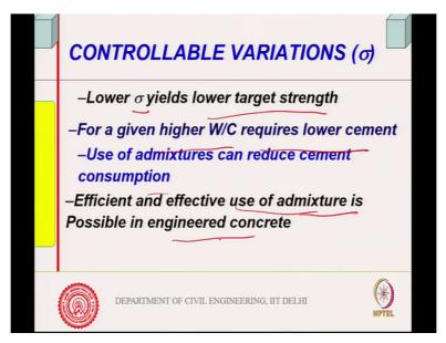
So lower standard deviation means lower target strength for given higher water cement ratio requires lower cement, that is what I was saying. Then use of admixture can reduce cement consumption, super plasticizers you know plasticizer super plasticizer, hyper plasticizers they can reduce and so therefore you can efficient and effective use of admixture is possible in engineered concrete. If it is manually mixed, you do not know how much quantity you are mixing.
