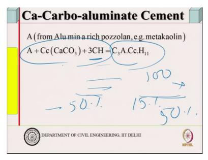
This is in plastic state and this will form solid product so you can blend cement through this system because cement will give you this and silica metakaolin may react in pozzolanic reaction, so some of these some of the additional silica if you have they can react with silica of the metakaolin react with like excess lime if it is there, so this is what it is.
