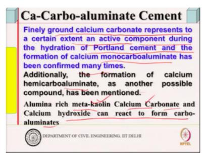
So, you have finely ground calcium carbonate presence to certain extent and active component during hydration of Portland cement. So this calcium carbonate some amount even if it is there in the cement system, it takes part in the reaction and forms carbo aluminates so formation of calcium mono carbo aluminate so this carbo aluminate is formed. So calcium heavy carbo is another possible compound so calcium carbonate also takes place in reaction forming calcium carbonate hydrate.
