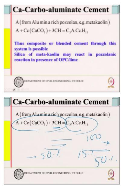
So, , this is the aluminum rich pozzolana metakaolin for example, this is this this is what it is calcium carbonate is written in this form CC. Calcium oxide is C, carbon dioxide is small c.
