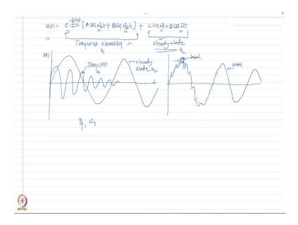
Now, I have an exponential term which is  $e^{-\xi\omega_n t}$  and this term is actually decreasing with time. I mean this whole term  $\left(e^{-\xi\omega_n t}\left[A\cos(\omega_D t) + B\sin(\omega_D t)\right]\right)$  is decreasing with time. So, after a certain amount of time this term would become 0. And as we said the term that vibrates at the frequency of the structure which in this case is  $\omega_D$  called the transient solution.
