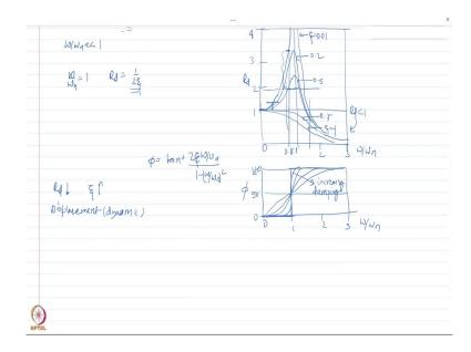
And, what happens to the phase angle  $\varphi$ . So, let us see here. So, when  $\xi$  equal to very small value or let us say it is 0. We saw that for undamped case it was let me first annotate the axis. So, this (vertical axis) is 0°, 90° and 180° this is phase angle  $\varphi$ , this is (horizontal axis) frequency ratio is 0, 1, 2 and 3.
