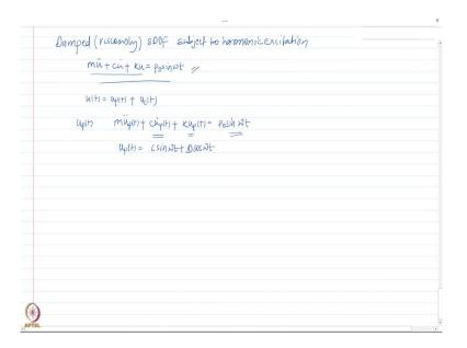
So, today what we are going to discuss damped or viscously damped system. Damped SDOF subject to harmonic excitation. Now, I am going to write down my equation of motion for this system.
