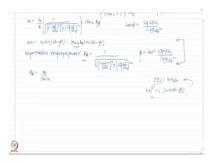
The deformation or displacement response factor  $R_d$ , as this expression right here-
