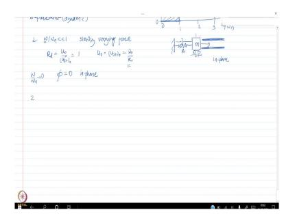
So, let us consider three cases. In the first case I would consider a case where  $\frac{\omega}{\omega_n} \ll 1$ . That means, this forcing frequency  $\omega$  is very small. Frequency small means what? It is a slowly varying load. So, I can say that it is a slowly varying excitation or force.
