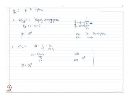
So, phase angle would become in this case 90°. If you substitute  $\sqrt[m]{\omega_n} \approx 1$  in denominator, it would be 0. So, it would be tan inverse of infinity which would effectively give you 90°. So, basically the applied force P(t) and u(t) they are out of phase by 90°.
