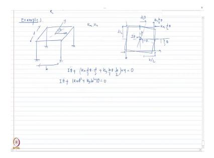
Then, see how do we tackle different problems. So, in example one here, what do I have here is actually a slab that is supported on 4 columns. The dimension of this slab is b in this direction and d along this direction.
