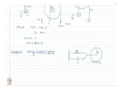
Now, let us see our example 5. In example 5, I again have a spring mass system except in this case I do not have a block but I have a rotational disc here. I need to find out what is the equation of motion, if there is rolling without slipping.
