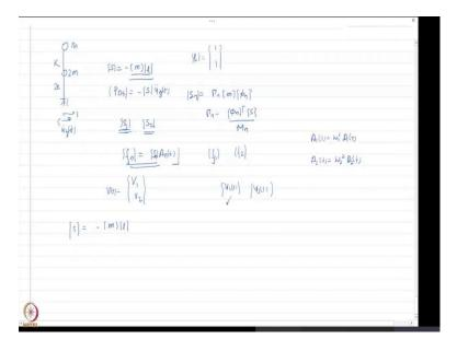
So, basically what I want to do here. We have masses 2m and m and stiffness 2k and k. If earthquake force  $(\ddot{u}_s(t))$  is applied let us say here something like this. I want to find out the expansion of the earthquake forces.
