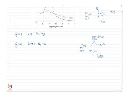
Now consider the other extreme case when  $w/w_n > I$ . What happens transmissibility ratio is actually approaches to 0 and in this case the total acceleration is approaching to 0. And that you can again imagine let us say I have a system and I have a very flexible column and, in this case, sorry the direction should be in this direction here.
