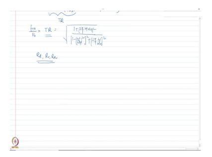
Which I can again write as here as ok and then I again have this term. So, this is my transmissibility ratio which is kind of another basically a factor to represent the effect of dynamic load.
