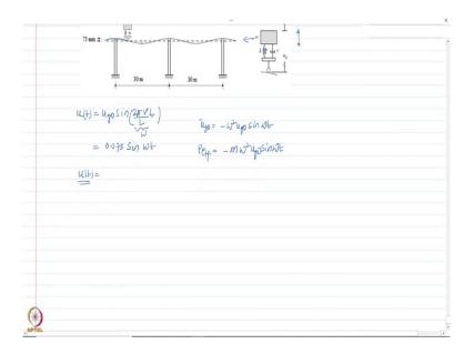
And because of movement in the horizontal direction, it would have vibration in the vertical direction we saw that it is because of the deck profile. So, we need to find out because of this movement what is the maximum possible force in the spring and the vehicle velocity at which that would occur.
