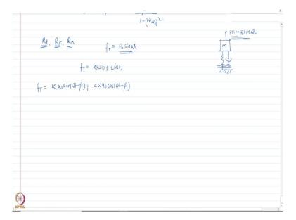
So, what are the response modification factor we have found out is  $R_d$ ,  $R_v$  and  $R_a$  which are basically for displacement, velocity and acceleration. And we did that because for some cases depending upon what kind of application that system has. You might want to find out what is the change in the displacement due to the dynamic excitation.
