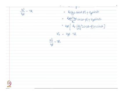
So, the maximum value of this one would be if you just consider the maximum just remove the t term here it would be this times TR. So, this is equal to the transmissibility ratio again
