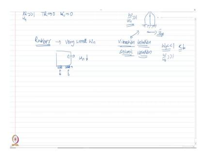
This is the principal behind vibration isolation ok and you would later see it could be simple vibration isolation of machines or it could be seismic isolation of structures as well ok. And the basic principle remains the same that the frequency of the structure is much much smaller than 1 or it is a very small value. So, that  $w/w_n$  is greater than 1 and you can imagine this happens frequency becomes very small when your stiffness is very small or it is a very flexible system.
