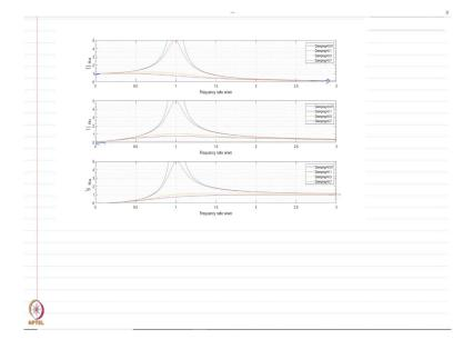
So, going to copy it here. So, if you look at it here, what do we see? We can see here this is my  $R_d$ , this is  $R_v$  and this is  $R_a$  and you can see the variation  $R_d$  starts with the value of 1 at a small value of  $\omega / \omega_n$  and then as the you increase the value it approaches to 0.
