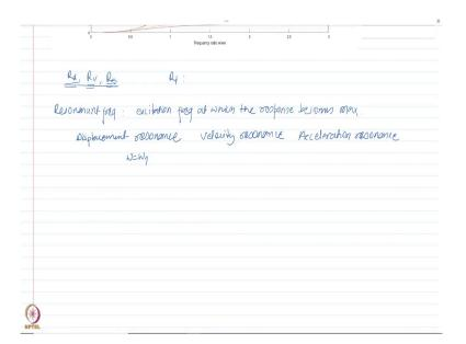
And remember we had used  $R_d$  to find out what would be the maximum response, you can use that. So,  $R_d$  is basically like an of a different value of frequency ratio what is the displacement. Now in this case we want to find out what would be the frequencies ratio at which these modification factors would have their peak values. Now remember the definition of resonance says or definite of definition of resonant frequency is the excitation frequency at which the response becomes maximum.
