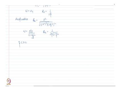
And if you do that, you will get excitation frequency, at the velocity becomes maximum is actually  $\omega = \omega_n$  and the  $R_v$  or the maximum value of the velocity response in terms of  $R_v$  is
