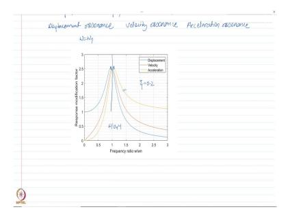
So, what I have drawn here on the same plot, in the same figure I have drawn 3 plots for the response modification factor of displacement, velocity and acceleration. So, using the expression for each of this I have drawn.
