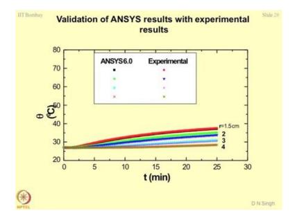
And, then if you match the results of ANSYS with the experimental studies where you are putting on y-axis the heat temperature and on the x-axis the time. So, for different radial distances you will notice that the experimental result and the ANSYS result they will be matching with each other. So, this gives more confidence in the type of exercise which is being done.
