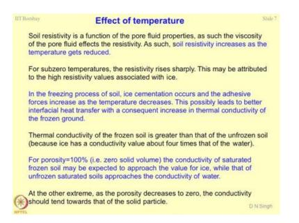
Effect of temperature. Now, what is going to affect the temperature maximum, raise or drop in the temperature? Again, is the pore fluid you agree or no?
