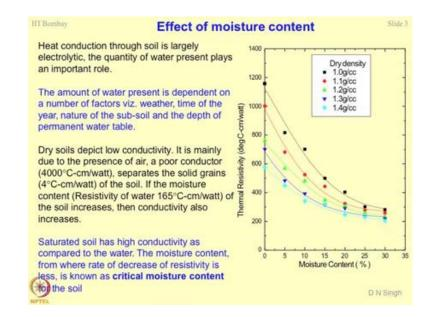
The second major factor which influences thermal resistivity is moisture content. So, what is the philosophy behind this type of mechanism? Why moisture content controls the resistivity? So, heat conduction is mostly through the pores or the pore solution which is present in the soil or the porous media. The reason is resistivity of minerals is very high as compared to the pore solution; so, most of the thermal conduction takes place either because of advection or because of advection.
