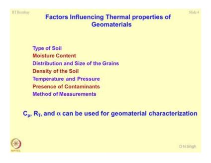
Let us talk about the factors which influence the thermal properties of geomaterials. The first one is of course, the type of the soil; whether a soil is a clay type of a soil, it is a sandy type of a soil; whether it is a rock material; whether it is a mixture of the combination of the two; whether it is saturated or not. So, moisture content becomes very important.
