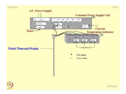
Now, this is the field probe, which was developed by my another student known as David; this is the one metre long field probe. This can be inserted into the soil mass and you can probe the temperature profile of the soil mass up to a depth of 1 metre. This is the electronic circuitry, which you have power supply, the timer, the constant power supply and the temperature read out units.
