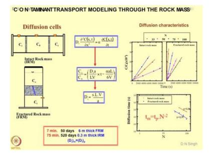
So, this type of diffusion characteristics you will be getting these are known as BTCs, break through curves, and if you plot normalized concentration with respect to time what you will notice is that the concentration keeps on increasing almost straight line with time, we have gone up to almost 1 lakh seconds or more than that and what we notice is a straight line portion. So, we stop the test over here.
