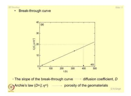
So, just to wind up today's thing this breakthrough curve which is nothing but a relationship between  $C_t/C_0$  and time in most of the situation this could be a straight line. We assume consider this steady state portion of the graph and for a given time you can work out  $C_t/C_0$ . So, if you know the initial concentration of the contaminant you can multiply it by  $C_0$  and you can get the  $C_t$  value. So, the slope of this curve will always give you diffusion coefficient.
