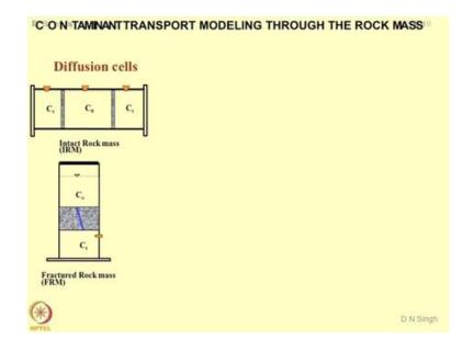
So, to study the contaminant transport modeling through the rock mass this type of a diffusion cell was fabricated, where it has three chambers and there are three top caps. So, in the middle of the chamber you can have fresh water and then these are the two samples of a geomaterial. So, you can take soil, you can compress it and you can make a pallet out of it or you can make a control volume which you can fix in the diffusive cell somewhere here.
