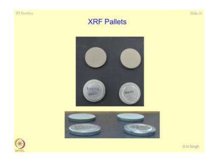
So, these are the pallets of X-ray. You can imagine a 0.5cm thick aluminum disk which is normally used. And half of this disk is filled up with cellulose state and the material for which chemical composition is to be obtained. And this makes a bond, you cover it apply some load, so that becomes a pallet and this pallet in this form goes in to the X-ray machine to get the fractions of oxides which are present in it.
