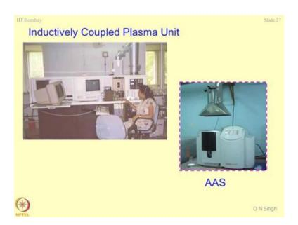
Now, this is the inductively coupled plasma unit, where you can find out the trace elements which are present in the soil mass up to the ppt level - parts for trillion (i.e., 1 in
