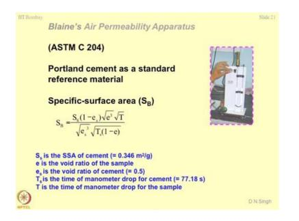
Now, this is the Blaine's permeability apparatus for finding out the specific surface area. Now, this is as per ASTM C 204 for admixtures and pozzolanic materials. And issue is that you use here as reference material the Portland cement. And for Portland cement the specific surface area is 3460 cm<sup>2</sup>/g. So, what do you think, that this method can be applied to any material or there are some constraints limitations?
