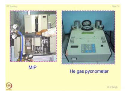
So, this is the MIP - Mercury Intrusion Porosimetry, you have already seen that helium gas pycnometer you have seen.
