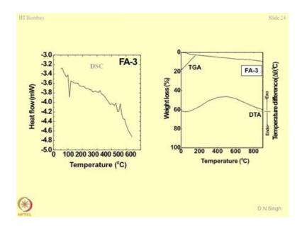
This is a good relationship which I wanted to show you which is response in a DSC. DSC also stands for doctor of science, highest degree in engineering or technology or any subject much higher than Ph.D. But here DSC corresponds to any guess Differential Scanning Calorimetry. So, what happens here is you heat the sample slowly and then try to see whether the heat flux is in the sample or out of the sample, again the same thing either exothermic or endothermic.
