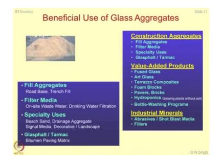
So, let us talk about now beneficial use of glass aggregates. So, glass aggregates are nothing, but you collect most of the glass either in the form of the bottle or the packing material, crush it and the heap of the crush glass will look like this; it is nothing, but shining sand particles.
