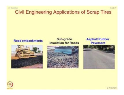
Some of the applications I have shown here for road embankments. So, you can stack them one over the other and then you can form embankment out of it; it is a good practice of creating embankments of the lagoons. So, you can put a layer of tires and cover it with the soil cover and this system can act as a embankment of sufficient strength. Sub-grade insulation for roads wherever you require insulation in the very hot and tropic countries this is where you can use as the sub-grade of the roads.
