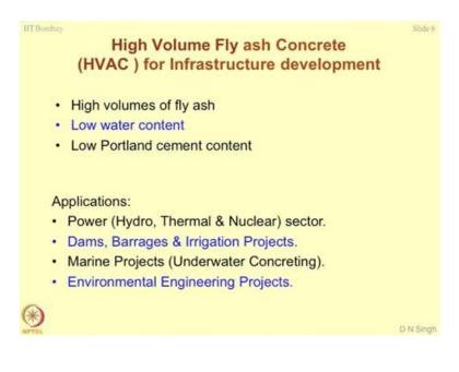
A good example of this type of construction for infrastructure development would be; any idea? Most famous application very recently which has been achieved Bandra-Worli Sea Link that is right. So, Bandra-Worli Sea Link is a good example of HVAC where high volume of ash has been used for increasing the durability of the concrete.
