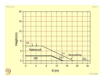
So, then what we did is we buried this coal residues use lot of native soil and made a carriage way for railways. So, these are the main and this is where the entire stability analysis was done, the idea wants to maximize the application of coal residues.
