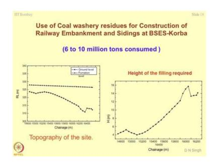
So, this is how 6 to 10 million tones of the coal residuals was used for making one embankment, and the height of the embankment was almost 16 meter 20 meter depending upon the different changes, this is the topography of the site you have RL in terms of the ground level and in terms of the formation of the level.
