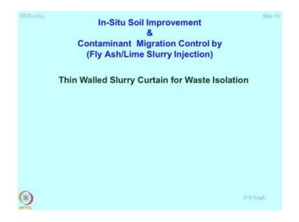
In-Situ soil improvement for which you can use fly ash slurry, mix with cement and lime and then you can inject it in the ground this forms a good gel and ultimately you can improve the soil.
