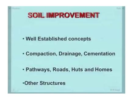
The second issue is Soil Improvement. The concepts of soil improvement are well established, what is the main idea of doing soil improvement? Should be good compaction, less drainage more cementation and so on. Where do you use them? For creating pathways, roads, huts and homes and sometimes other structures also which are of strategic importance. So, what is the challenge in soil improvement? To avoid?
