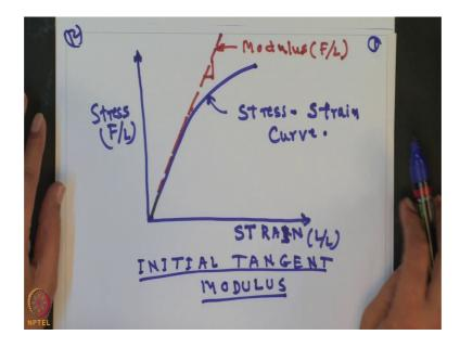
You can draw a relationship between the stress that is F by L in the x axis; y axis and the strain this is L by L in the x axis. So, this nature of the curve let us say stress strain curve of geosynthetics material is like this. So, these are the stress strain curve ok; so, from this stress strain curve; we want to determine that, what will be the initial tangent modulus. So, if we can draw a straight line from the origin tangent to the circle and the slope of
