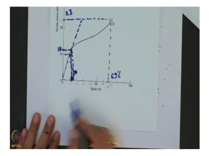
So, let us say this is the, this the non woven geotextile material whose tensile stress and strain curve is looks like this. And these material have some thickness and this material have some mass per unit area.
