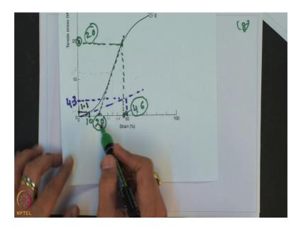
Now, I will give the another example for a non woven needle punched geotextile material. For example, this is the tensile stress and strain curve for the non woven needle punched geotextile material; this is non woven needle punched geotextile material and this material I say that it is non woven needle punched geotextile material.
