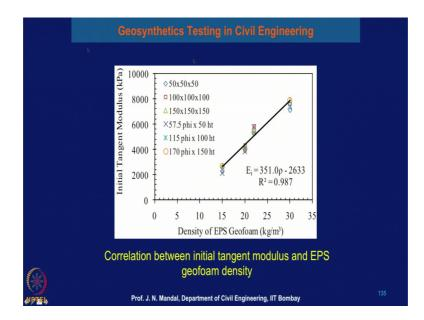
I will now, show you a relationship between the EPS geofoam and the tangent modulus. So, here this diagram show the correlation between the initial tangent modulus and EPS geofoam block.
