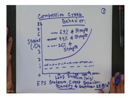
That it call the compression creep behavior. So, compression creep behavior of the geofoam is very interesting and if you know the compression creep of the EPS geofoam, so you can design that what should be the thickness of the EPS geofoam material. But these test is very long term testing and this is time temperature superposition, and it takes long time to perform this kind of compression creep behavior of the EPS geofoam material it may be 100, 1000, 2000, 5000, 1 lakh minutes.
