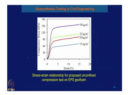
You can see this is the compressive stress and this is the strain and compressive strain is in terms of kilopascal and this is the stress and strength relationship for the proposed unconfined compression test on EPS geofoam. So, you can see these one for a particular density of 15 kg per meter cube, then 20 kg per meter cube, 22 kg per meter cube and 30 kg per meter cube.
