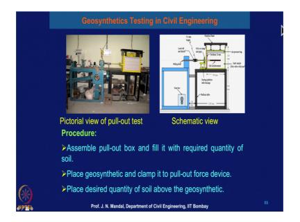
So, this is the pullout test equipment and this you are pulling, of this shear you can see some schematic diagram. And here I am showing you here is that here is the box, pull out box and is rest on a platform with the bearing and you are to provide with some kind of the airbag also top of this.
