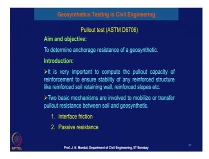
So, two basic mechanisms are involved to mobilize or transfer the pullout resistance between the soil and geosynthetics you want be the, what is the interface friction and what should be the passive resistance.
