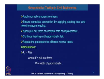
So, from this test you can calculate that what should be the pull out force that is P of r. So, that will be the what will be the pull out force that is F and what will be the width of the geosynthetic material. So, you can calculate that P r will be equal to, so P of r you can calculate that P of r will be equal to F divided this W, where F is equal to pull out force, F is equal to pull out force and W is equal to width of geosynthetics, width of geosynthetics material.
