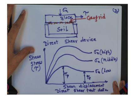
So, this geogrid attached to the block, this geogrid attached to this block then you are applying load and then you are giving the shear stress and bottom on is the soil. So, this is the direct shear device. So, any kind of the material we can determine what should be the friction angle between the soil and the geogrid or between the soil and the geomembrane or between the soil or any concrete woven geotextile and nonwoven geotextile material.
