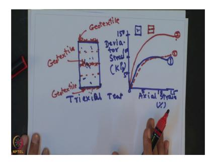
So, you will perform the tri Triaxial Test. So, these triaxial test are to be confirmed and there is a beneficial effect of geotextile when you place the geotextile material at the proper location. Now, you take some 2 or 3 test on the then, sand sample and at a confining pressure, you can give confining pressure 21 kilo Pascal or 210 kilo Pascal for different soil and geotextile configuration.
