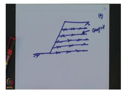
So, you can place the number of the layer of the geogrid material. So, these are all this geogrid material ok. You have place one layer in between the foundation and the embankment soil. So, this is the geogrid material. So, here geotextile material act as a tension or geotextile material act as a membrane type of the reinforcement.
