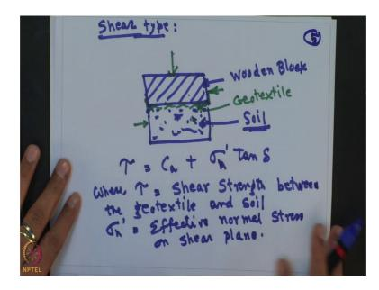
Now, geosynthetic material also acts as a shear type. So, far we mentioned about the reinforcement in membrane type, now we will discuss the shear type. Now, at shear we perform the test in a direct shear test. So, you can have a better visualization by the direct shear stress. You know what is direct shear test and you know how to perform this shear strength of the soil; then, we will perform how we can perform this shear strength of the geotextile material.
