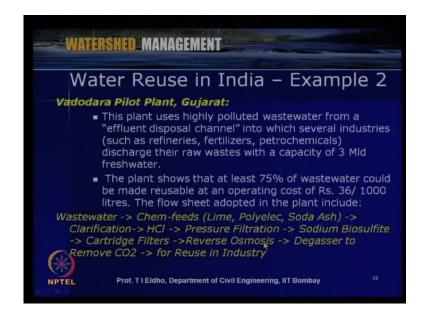
This is example one and in second example here another Vadodara pilot plant in Gujarat. So, this plant uses highly polluted wastewater from a effluent disposal channel into which several industries such as refineries fertilizers petrochemicals discharge their raw wastes with a capacity of 3 million liters per day freshwater.
