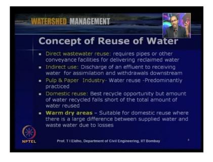
Direct wastewater reuse requires pipes or other conveyance facilities for delivering the reclaimed water. So most of the time we need the dual say system where the reclaimed water another piping system through which we can sent this reclaimed water so that is for direct wastewater reuse so that may be for irrigation or agriculture or flushing or maybe some of the industrial processes.
