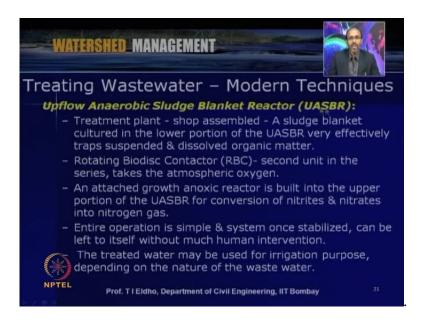
Then say, let us now look into some of the modern techniques used for treating the waste water so this is mainly say, we use as tertiary treatment so first one is the up flow anaerobic sludge blanket reactor or UASBR so here treatment plant say, we can would have say, actually as module it be available and directly it can be obtained from the shops and it can be assembled a sludge blanket cultured in the lower portion of the UASBR very effectively traps suspended and dissolved organic matter.
