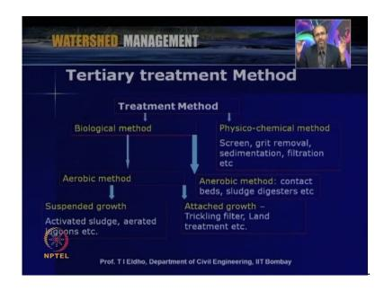
So, that way when we look into the tertiary treatments so we can classify the treatment method into the biological methods and physico-chemical method as far as physicochemical method is concerned like a screen grit removal sedimentation filtration etcetera so these are all physico-chemical methods
