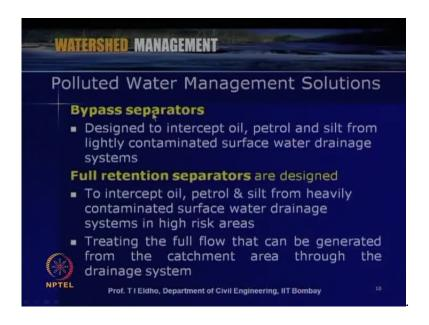
And then third solution is polluted water management solution so here say, we can have bypass separators like designed to intercept oil petrol and silt from lightly contaminated surface water drainage systems
