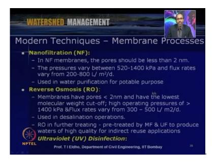
Third system is so called Nano filtration so here in Nano filtration membranes the pores should be less than 2 nanometers so the pressures vary between 500 and 20 to 1400 kilopascal and flux rates vary from 200 to 800 liters per meter square per day and this the water passing through the Nano filtration we can directly use for even for portable purposes like recharging or other kinds of purposes.
