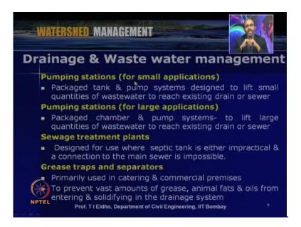
Then Now, second one is drainage and waste water management so here say, the water say, which we are draining that we are trying to use effectively so we can have pumping stations say, for example for small applications like a packaged tank and pump systems designed to lift small quantities of a waste water to reach existing drain or sewer
