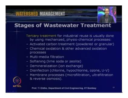
So, when we look into tertiary treatment actually say, when we look into the waste water so the tertiary truth after the tertiary treatment the water can be used for various purposes in say, reuse is concerned or recycle after the recycling through the tertiary treatment we can directly utilize like for irrigation then say, toilet flushing or direct industrial purpose like that
