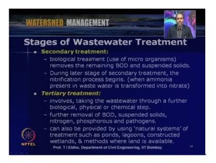
Then next one is the secondary treatment so here we can go for various kinds of treatments like a biological treatment say, for example to remove the microorganisms and removes the remaining BOD and suspended solids so here during later stages of secondary treatment the nitrification processes like when ammonia present in waste water is transformed into nitrate
