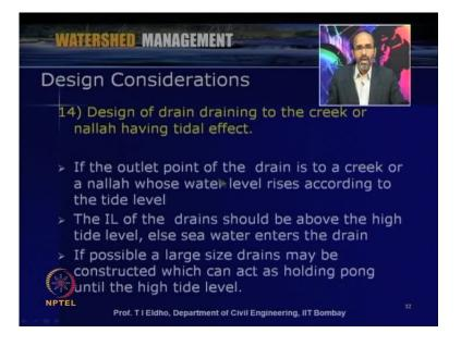
Then connection between the main drain or either side of the road, we have to see. Then, points, important points like design of draining to the creek or nallah having tidal effect. So, as I mentioned in a city like Mumbai, tide is an important factor as far as flooding is concerned.
