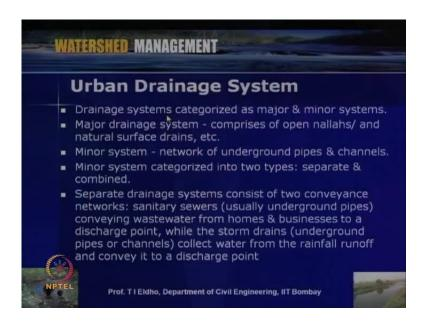
So, now, let us discuss about the urban drainage system. Since drainage pattern or appropriate drainage is given, then to a biggest, the urban flooding can be reduced. So, appropriate urban drainage system very important as far as, the, the urban flood management is concerned. So, urban drainage system, drainage system generally we can categorize into major drainage systems and minor drainage systems.
