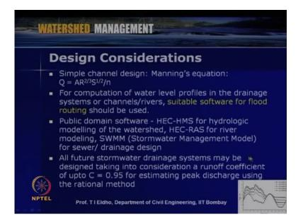
And then, hydraulic design - just like the cross section of the drainage system. We can use simple equations like Manning's equation or Chezy's equations for simple design.
