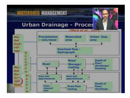
So, as far as urban drainage system is concerned, there can be major drainage systems or the minor drainage systems. So, when we look into the urban drainage processes, so we can put it in a flow chart like this. (Refer Slide Time: 18:05) So, the urban runoff is coming from precipitation or snow - precipitation as rain or snow - and then, if you consider the watershed area, there some area will be pervious area and some area will be urbanized or impervious area.
