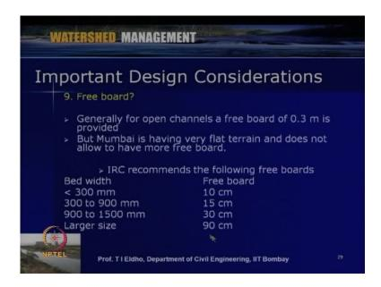
So, as far as IRC 50 code, minimum longitudinal gradient is 0.3 percent. Then free broad also we have to when we go for open channel type design, 0.3 meter is the prescribed
