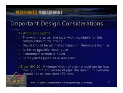
Then another important aspect is width and depth. So, the width is as per the local width available for the construction of the drains; then depth should be estimated based on Manning's formula. As far as possible, we can go for rectangular drains. Then economical section is the width is equal to 2 times depth, and some places, we may have to if we are going for open drains; some places we may have to go for further pipe drains.
