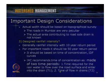
So then, actual width should be based on topographical survey; then the roads in Mumbai for example, we have to see the actual area contributing to road side since it is heavily populated, and then, the roads are very narrow. So, that way, we have to consider.
