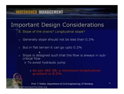
Then eighth point is slope of the drains like longitudinal slope. Generally slope should not be less than 0.3 percent, but in flat terrain it can go up to 0.2 percent, and slope is designed such a way that the flow is always in subcritical flow. So, there should not be any supercritical flow condition so that there is any hydraulic jump can takes place. Within a channel, that may create further flooding problems.
