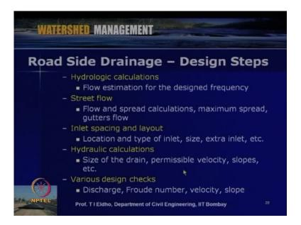
So, the final layout, we should have like all ditches, waterways, inlets, manholes, mains, laterals, culverts, flow direction, Etcetera. So, we have to go systematically. Then, next step is hydrologic calculations. So, we have to identify as far as roadside road is concerned, so how much water will be coming from both sides. So, we have to see that area and then how much is a rainfall possible.
