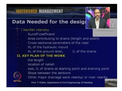
Then we need a large quantity of data when we go for the road side drainage system design or the urban drainage design. So, some of the important data like rainfall intensity, then runoff coefficient, area contributing to drains, then cross sectional parameters, the reduced level of the hydraulic mount, then reduced level of the ground level, invert level of the drains. So, like this, all this data required as far as the drainage design is concerned.
