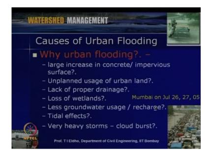
So, some of the causes of urban flooding, say here I have mentioned. So, it can be, as we discussed - a large increase in concrete in impervious surfaces or unplanned usage of urban land or lack of proper drainage or loss of wet lands or it can be less ground water usage or recharge tidal effects or very heavy storms or cloud burst or say like a climate change effect.
