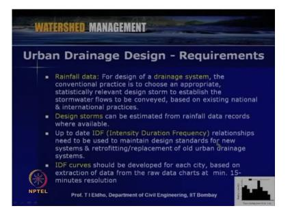
Then, as far as rainfall is concerned another important data. So, for design of a drainage system, the conventional practice is to choose an appropriate statistically relevant design storm to establish the storm water flows to be conveyed based on existing national and international practices.
