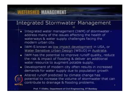
Let us look into what is integrated stormwater management. It is actually integrated water management only or IWM of stormwater. This addresses many of the issues affecting the health of waterways, water supply challenges facing the modern urban city. When we are effectively utilizing the water at local level wherever the stormwater takes place, we are actually reducing the water related problems, since we will be recharging the water or storing at local level. That can be directly utilized.
