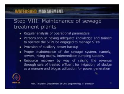
Then step number eight - maintenance of sewage treatment and plans. So, we have to see that regular analysis of operation parameters are done so that, the, we keep the strict maintenance of the treatment plants. Then persons should have adequate knowledge and we have to train to operate the sewage treatment plans, and then, there should be provision of auxiliary power backup; then proper maintenance of the sewage system namely: sewers, rising mains, intermediate pumping stations.
