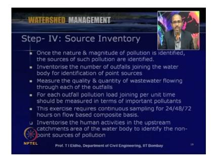
Now step number 4 is related to the source inventory. So, once the nature and magnitude of pollution is identified, the sources of such pollution are identified. Then in inventory we have to make an inventory of the number of outfalls joining the water body for identification of point sources.
