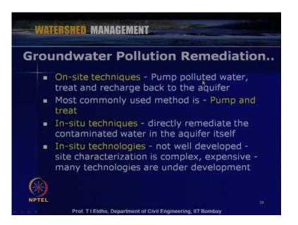
As I mentioned here on-site techniques, we generally pump the polluted water, treat and recharge back to the aquifer systems. So, one of the most commonly used methods are pump and treat. So, we pump the polluted water, treat it and either use it or put it back. In in-situ techniques, we directly remediate the contaminated water in the aquifer itself. In in-situ technologies, we do not know the actual total groundwater system or subsurface system, so that way it is called as complex process.
