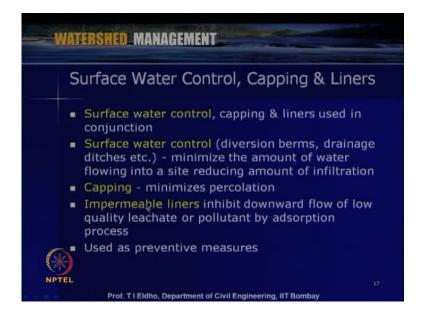
Some other techniques like surface water control, capping and liners. So, these are also used in many countries for the groundwater protection or groundwater pollution control.
