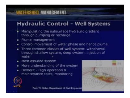
Another commonly used technique is called hydraulic control. As shown in this slide, we are manipulating the subsurface hydraulic gradient through pumping or recharge. For
