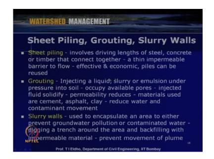
Some of the other techniques is used are sheet piling, grouting and slurry walls. Here, this sheet piling involves driving lengths of steel or concrete or timber that connects together a thin impermeable barrier to flow. So, this is effective and economic. Piles can be reused, so we can control the movement of the pollutant. Grouting means injecting a
