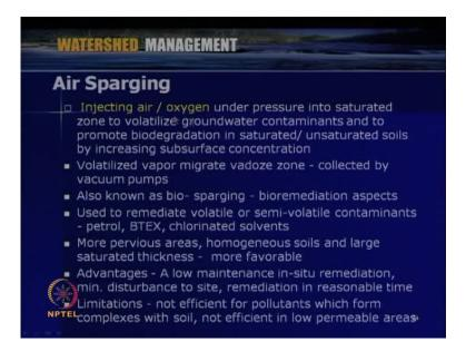
Another commonly used methodology is called air sparging. Here, what we do is we inject air or oxygen under pressure into saturated zone to volatilize the groundwater contaminants and to promote biodegradation in saturated or unsaturated soil by increasing subsurface concentration. Generally, this air sparging can be used for volatile organic contamination. The volatilized vapor migrates through the vadoze zone or the unsaturated zone and the vacuum pumps collect these.
