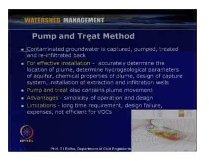
As I mentioned, one of the most commonly used treatment technology is on-site technique of pump and treat. So, what we do is the contaminant plume, wherever it is there in the hot spot, through boreholes or through wells, we pump this polluted water out of the aquifer systems. We treat it outside depending upon the contamination and then we can either pump it, recharge back to the aquifer system or we can use it or we can spill it to the nearby sources surface water sources.
