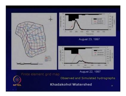
So, here, you can see in this slide, the gridding is shown here. So, this is the major channel within the watershed. So, accordingly, according to the slope of the, say within the watershed, so, we have made a strip. So, you can see that various strips coming say joining to a channel. So, these are the strips.
