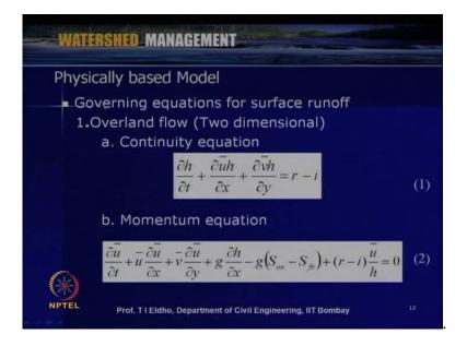
So, the governing equations here, in this slide, I have kept. So, here, overland flow if we are doing two-dimensional modeling, the continuity equation is given by this equation - del h by del t plus del u bar h by del x plus del v bar h by del y is equal to r minus i - where h is the depth of flow and u bar is the velocity and v bar is the velocity u in x and y directions, and then, r is the rainfall intensity and i is the infiltration rate.
