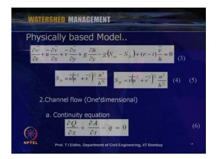
So, for one-dimensional channel flow modeling, we have to solve the continuity equation and the momentum equation. So, continuity equation is given by del Q by del x plus del A by del t minus q is equal to 0 - where Q is the discharge; t is the time; A is the flow cross section area small; q is the overland flow component coming to the channel and that we have to route, and the momentum equation one dimension is shown by this equation number 7.
