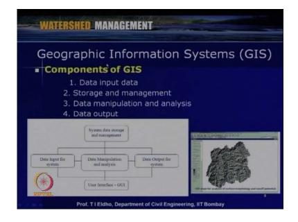
So, that way, the important components of GIS have the data input, then storage and management data manipulation and analysis and the data output. So, this shows a typical
