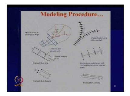
So, the modeling procedure again I will describe by using a figure. So, here, you can see that if this is our watershed which we consider, so, this is first we delineated the watershed and this is the area which we consider. So, this is the major stream and then minor channels or the streams coming to the major streams.
