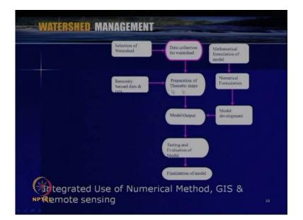
So, here, depending upon the requirement, so, these are the steps the flow chart which I mentioned. So, here, starting with the various database development, model development, and then evaluation and finalization of the model, and then, if you are going for rainfall runoff modeling, we can decide the infiltration models which we are going to use various models are available as we discussed earlier.
