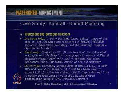
So, including the drainage slope map, land use land cover map, and the digital elevation model, so, this shows the drainage map for the Khadakhol watershed So, the drainage map as far as data-based preparation, the various steps here I have mentioned. So, the drainage map initially we scanned the topographical maps of the area which is in 1 is to 25000 scale.
