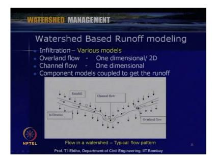
So then, as I mentioned say at IIT Bombay, we developed a model physically based model for rainfall runoff modeling for watersheds. So, the details we are going to discuss in the coming few slides. So, here, we developed the one-dimensional models, steep based model for overland, and then, channel flows, one-dimensional diffusion wave based and overland flow as kinematic wave based model.
