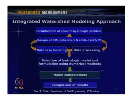
So, here, I have shown a flow chart where how we can do integrated watershed modeling approach. So, first step is we have to identify the specific problem; it can be hydrologic problem or it can be soil erosion problem or sediment yield problem or whatever problem which we are trying to do as far as the watershed is concerned so that we can identify, and then, for any of these kinds of studies, we need good amount of data.
