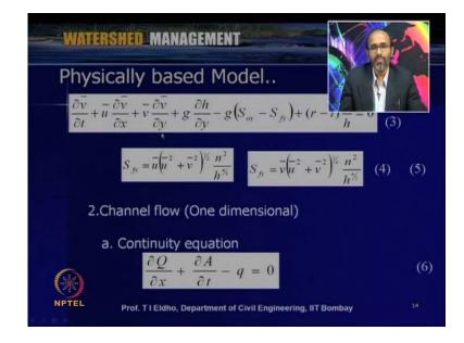
And this energy slope – here, we can use the Manning's equation as given in this equation number 4 and 5. So, that way, say these equations if we are going for twodimensional modeling, we can directly solve these equations and then we can get the output will be the depth of flow at particular location and the velocity is in x and y direction at the at particular time step or particular location, and then, channel flow is concerned, as I mentioned generally we can go for one-dimensional modeling.
