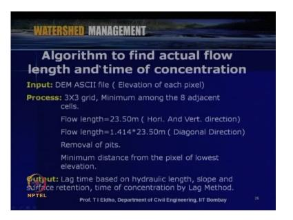
So, now say, the algorithm to find actual flow length and time of concentration. So, input is as I mentioned, we give it as digital elevation model in ASCII file. That means, elevation of each pixel and process is 3 by 3 grid, minimum among the 8 adjacent cells and flow length is 23.5 metre, horizontal and vertical direction and flow length is 1.414 into 23.5 diagonal direction.
