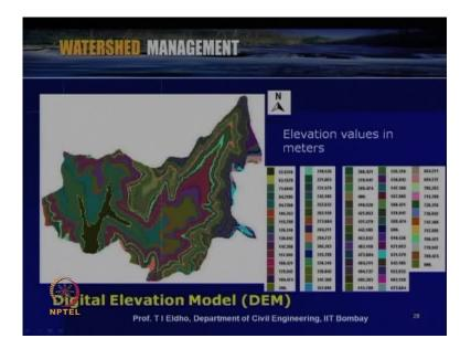
So, then using this specified procedure, we have generated a digital elevation model. So, this shows the digital elevation model for the Amba watershed. So, elevation values are listed here in metres. So, the elevation varies from 52.6 metres to 800 metres above the mean sea level. So, this is the digital elevation model for the Amba watershed.
