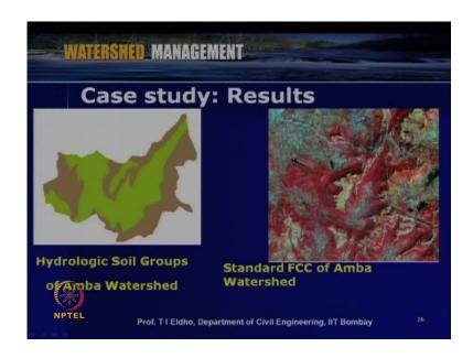
So, based upon all this available data, within the GIS environment, here, we used the GRAM plus plus package, which belongs to IIT Bombay. So, based upon various data available toposheet, the remote sensing data and then various field information, we have generated various maps within the GIS environment.
