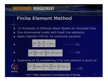
Then the next method I would like to discuss briefly is so-called finite element method. So, here we again use the kinematic and diffusion wave forms of overland flow to demonstrate the finite element scheme. We have already seen the governing equations as far as the kinematic wave scheme is concerned. So, the continuity equation and the momentum equation, momentum equation, kinematic waveform is S 0 is equal to S f.
