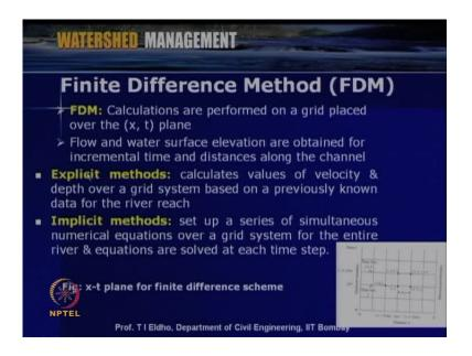
Now, let us see some more aspects about these two techniques: finite difference method and the finite element method. As I mentioned already, in finite difference method the calculations are performed on a grid placed over the domain. so if it is 1 dimension, it can be x t plane; or in 2 dimension it can be x y t plane; or in 3 dimensions it can be x y z and t plane. This is for example, in 1 dimension explain and t.
