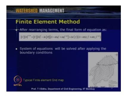
He used implicit finite difference scheme as we mentioned here. So, the final system of equation is given here and then after rearranging the term we will get a finite system like this. So, here if you are using the say in Crank Nicolson scheme, here omega will be 0.5 and in this scheme we apply the boundary conditions and initial conditions and then we can solve the system of equations.
