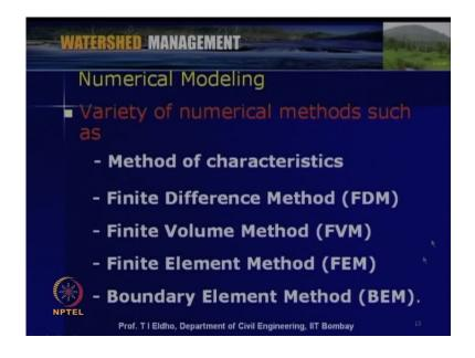
So, some of the important numerical methods I have listed here like a method of characteristics, finite difference method, finite volume method, finite element method, boundary element method and now, latest study is mesh-free methods.
