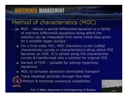
So, for example, for a first order partial differential equation m the method of characteristics discovers curves so-called characteristics curve or characteristics along which partial differential equations become ordinary differential equations. So, we do certain transformations and then accordingly we do so then it is sold along the characteristics curves and transformed into a for original partial differential equations.
