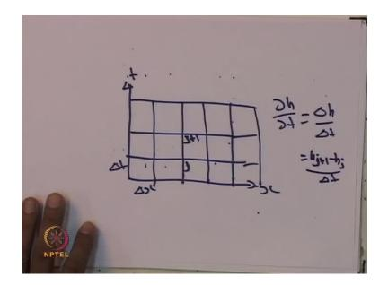
So, here again you can have this is x this is t so we can consider the variations with respect to the x t plane so that is x plane give the variation in space and this t represent the time so this will be now delta t and this will be delta x so that way we can consider. So, we can then represent delta h by delta t with respect to if we consider this as j and this is as j plus 1 so we can write with respect to h j plus 1 minus h j divided by delta t.
