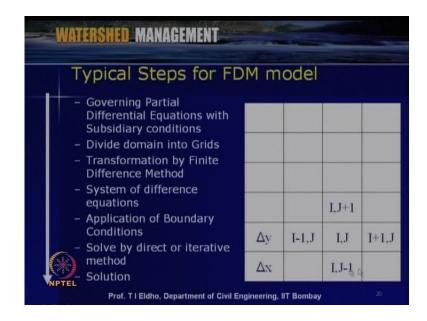
In finite difference method we can typically follow step by step procedure. So, for the given governing partial differential equations, the boundary conditions, we can divide the domain into grids as shown here and then put the nodal junctions at grid. These junctions we can identify various values like a I minus 1 j or I j; this we can write 1 2 in row-wise and 1 to end the column-wise also.
