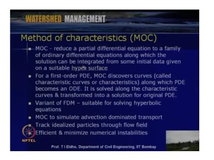
So, then another important method which we use in water resource is so-called method or characteristics so method of characteristics is also one variant of finite difference method so here the method or characteristics here in this slide you can see the details are given MOC reduces a partial differential equation to a family of ordinary differential equations along which the solution can be integrated from some initial data given on a suitable hyper surface.
