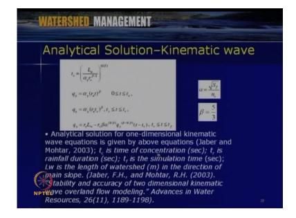
Now coming back to the watershed modeling, for example, if we consider the kinematic wave form of the Saint-Venant's equations, as I mentioned, we can either go for the analytical solution., so here the analytical solutions for 1 dimensional case, I have given as given by Jaber and Mohtar as published in Advances in Water Resources in 2003.
