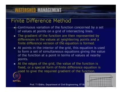
Then we have to consider the governing equations; so here, if this is x so, for 2 dimensional modeling, x y so this is delta x, this is delta y, so that way we will do a discretization and then the gradient of the function are then represented by differences in the values of at neighboring point s and a finite difference version of the equation is formed.
