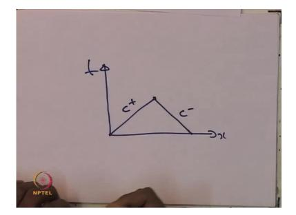
For example, this is an x t plane then we can consider we do some transformation so and then we will be having a c plus or c minus characteristic lines or characteristic curve and with respect to that the approximation will be done.
