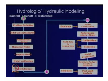
Here in this slide for example,, when we consider watershed based modeling rainfall to runoff, so here various steps I have identified in this slide. As I mentioned, the problem definition that means, if the objectives, depending upon the objectives we can define the problem and then we can go for the solutions.
