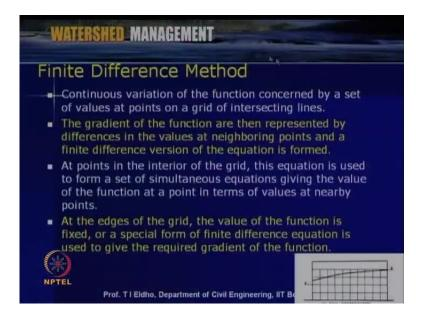
So, first one is the finite difference method; here what we do the finite difference method is concerned, the continuous variation of function concerned by a set of values at point on a grid of intersecting line. So, if this is the domain, we discretize this domain into rectangular or square grids like this and then we use the governing equations, so that we discretize the governing equations.
