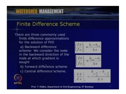
So far as the finite difference scheme is concerned, generally 3 schemes are available which are commonly used. First one is called backward difference; backward difference means for example, if we consider del h by del x, so here we consider the node in the backward direction of the node at which gradient is sought.
