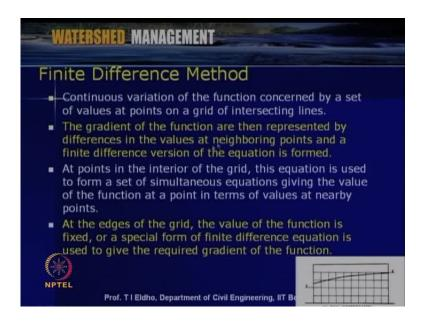
So, these details we will discuss further so finally at the points in the interior of the grid this equation is used to form a set of simultaneous equations giving the value of the function at a point in terms of values at nearby point. So, we can see that nearby points once we consider this particular point the nearby points with respect to nearby points we can use various schemes like backward forward or central difference schemes so that finally we can form a system of equations.
