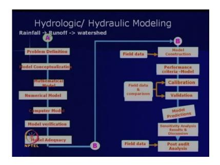
Field data like a rainfall pattern rainfall intensity or the various watershed parameters like size of the watershed land use, then Manning's roughness coefficients, then the saturated hydraulic conductivity, etcetera. So, the field data is required to construct the model. This model construction means the model which we are to construct for the particular watershed, to deal with the particular objectives which we have said.
