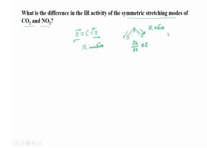
So let us look into the next question, what is the difference in the IR activity of the symmetric stretching modes of CO 2 and NO 2. So we discuss in the class this carbon dioxide the symmetric stretching mode is both the CO bonds are either lengthening or their contracting at the same time. So because this is a linear molecule there is no change in dipole moment with respect to the displacement from the equilibrium bond length.
