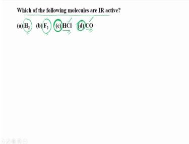
The first question we have is which of the following molecules IR active. So we have 4 choices H 2, F 2, HCL and CO or carbon monoxide. So, as we can see H 2 and F 2 they are homonuclear diatomic molecules on the other hand, HCL and carbon monoxide hetero nuclear diatomic molecules. So, we know so, HCL and CO they will be IR active. So, the right answers are c and d.
