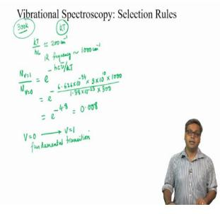
Let us say 300 Kelvin the thermal energy at room temperature is given by kT. As IR spectral transition is commonly reported in wave numbers the thermal energy is approximately kT / hc. And if you put the values here then what we will get is approximately this is 200 wave numbers but most vibrational wave numbers are significantly greater than 200 wave numbers or in other words this IR frequency in wave numbers we can say there in the order of thousand wave numbers.
