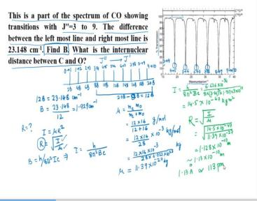
So, let us look into the problem here is a real rotational spectrum of carbon monoxide. On the x axis, we are plotting wave number or centimeter inverse. On the y axis, we are plotting percentage transmission. So, at whichever wave number there is some absorption of light the percentage transmission is not 100 or in other words, in these wave numbers, the percentage transmission are less or much less than 100.
