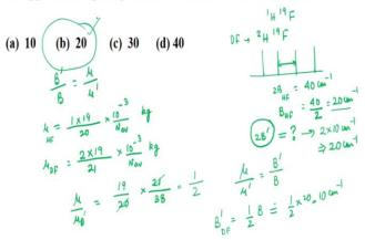
So the first question we have is the spacing between the rotational lines of HF is 40 wave numbers and the question is what is the approximate spacing between the rotational lines of DF in centimeter inverse. So, HF we can write H that atomic weight 1 fluorine atomic weight 19 and DF. So, D is an isotope of H, because I can write DF as H with atomic weight to 19 F. So, the question is for HF, I have a rotational spectrum and the spacing between the lines that is 2B for HF = 40 wave numbers.
