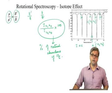
So, now, let us look again at the experimental spectrum, we see as the value of J increases the gap between the isotopically substituted line and the other line that is between C 13 and C 12 increases from what we had at lower J values. So, we can now explain the isotope effect from the experimental spectrum of carbon monoxide. So, we can find that B and B prime from the experimental spectrum. So, which will also provide us with this ratio B prime / B or we can also find B / B prime.
