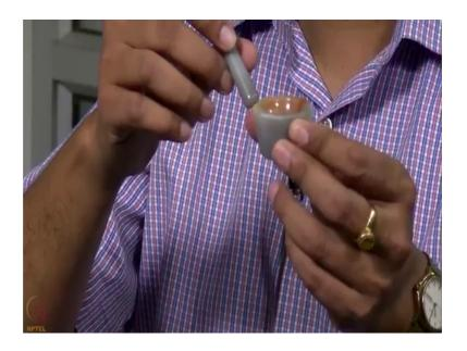
This is agate mortar and pestle which is made up of a stone and this stone is very hard for when we grind the sample here. This does not make any scratch on the stone and no sample gets stuck to this stone, during the sample preparation process. So, once we have powder the sample using this mortar and pestle.
