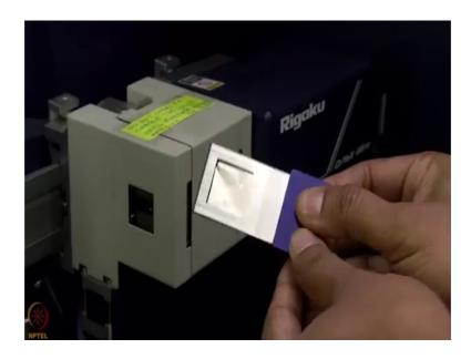
This nickel filter is used to remove the k beta component of the copper radiation and one reaches the detector is just the copper k alpha. So, this diffractometer works in a theta
