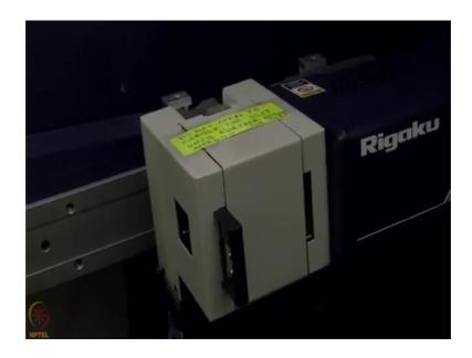
On the detector which is be written Rigaku at the back that is the detector for X-ray here. So, before this sample before the X-ray beam it goes to the detector we have a beam stop here. That beam stopper stops the direct beam from going to the sword going to the detector. Because the direct beam is very high intensity and it may spoil the detector and that is why we should have a beam stop. So, in this X-ray tube we need to pull the anode which is at the back of this tube.
