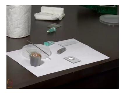
So, what we will do on the diffractometer is we will place this sample in front of the X-ray beam. And then we will make the sample rotate like this at one hundred and 20 RMP so that the entire sample leaves you evenly exposed. Because the beam that we have here is a line focus, which means the beam is like a line which is like this. And then if we rotate this sample we have below the beam the entire sample gets exposed to that beam.
