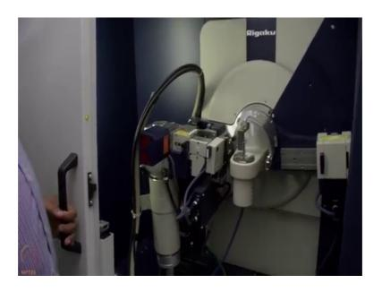
Are the equipment with the X-ray tube detector and the sample stage? On the left hand side here we have the X-ray tube mounted. This is mounted from top and you can probably see that this is a copper based X-ray source which is written here as copper.
