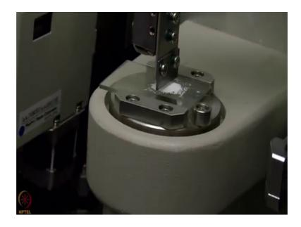
So, this sample is now placed in the middle portion if we see that here at this point the X-ray beam will come and heat. As a result if we will rotate the sample during the measurement it will expose the entire sample to the beam. So, we need to close the door because we cannot run X-ray diffractometers with the doors open for safety reasons. We should not be exposed to these x rays during the experiment.
