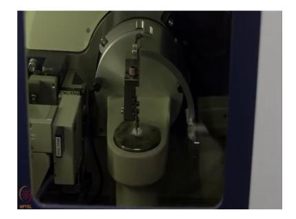
So, here you can see that during the measurement the sample is rotating at 120 RPM on the sample stage. And the data is getting recorded on the computer which is going to be shown.
