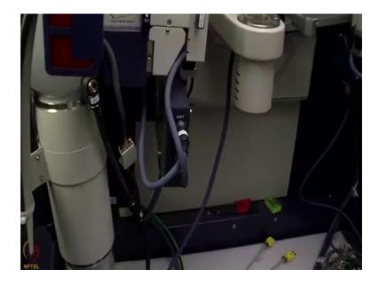
In this case this works on a theta theta geometry. So, I have the X-ray beam coming from my right hand side and the detector is on my left hand side and during the measurement both the detector and the source goes up slowly. So, this is called the theta theta geometry. The other geometry that is possible is a theta 2 theta geometry.
