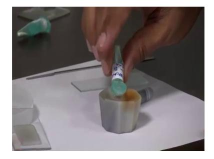
To make the sample we transfer the cystallized material, it may be nice crystals. So, this is a poly crystalline powder.
