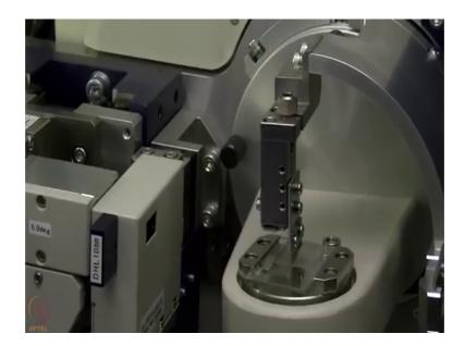
This is the sample stage which can be rotated like this during the experiment it rotates which then makes the sample uniformly exposed to the beam, and it removes all possible preferred orientation effects. The X-ray beam comes from the left hand side, gets diffracted from the sample placed on this plate here. And then gets diffracted and gets recorded.
