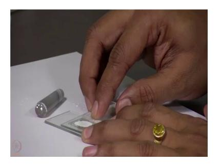
So, now what we need to do is to bring the sample to the center, because we do not have large amount of sample we have made a heap at the center. And then we need to make it flat from the top using a glass plate. So, that the top surface is flat and the sample is uniformly spread in the center. So now, this sample is ready for recording powder X-ray
