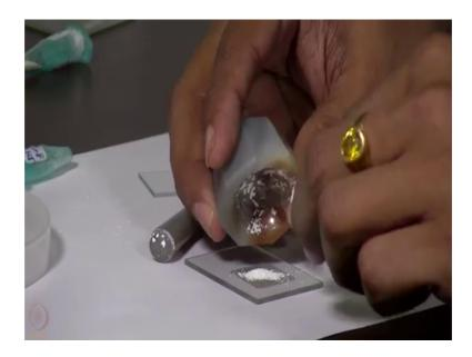
We can scratch it further to take the remaining amount of sample that is there inside the mortar and pestle this mortar.
