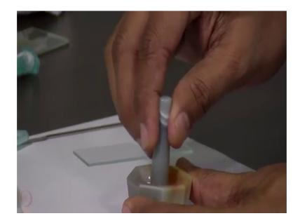
This grinding should be done very carefully and harsh grinding may lead to conversion of the sample to a different form. In case the sample contains some solvent it may so, happen that during this grinding if we apply too much of pressure the solvent can evaporate and lead to a different crystal structure than the starting material.
