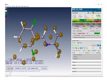
So, after selecting those hydrogens and marking those atoms and marking them as hydrogens if we tried to refine, we will see that the R factor reduces. You do it a few times till you reach a convergence so, all these weighing parameters should become green which would indicate that the refinement is reaching convergence.
