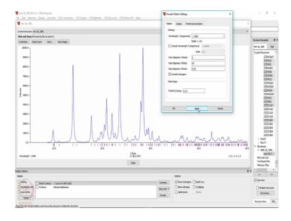
But the same if we use copper 1.5406 angstrom wavelength and then we apply it you see that the peaks are well spread, they are not merged and with the same FWHM there are several peaks which can be distinguished from the other. All these peaks completely disappeared or merged through a wavelength.
