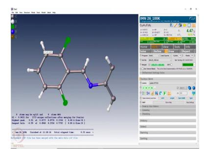
And then at this point we remove all the other residual densities and let us bring the cursor at the bond between carbon and hydrogen it shows the distance.
