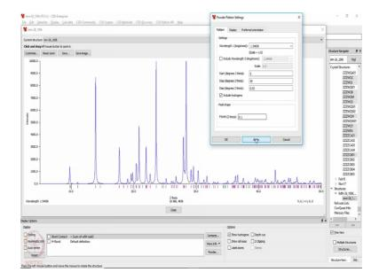
To be able to a correctly compare or accurately compare, you can go and customize, you can increase the FWHM to about 0.25, which is a generally case for routine data collections. And see here this is determined using the copper k alpha radiation.
