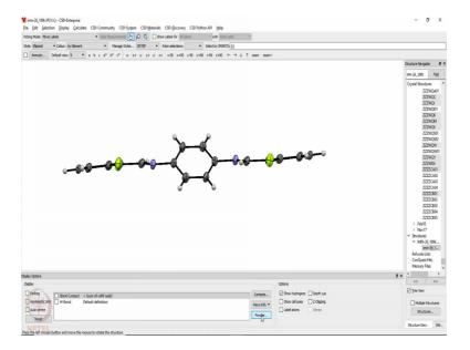
So, now this is the (Refer Time: 21:42) here the structure that we have solved from a single crystal x ray diffraction data. What else we can do with it, see a single crystal is grown from a starting bulk material that was a polycrystalline powder to start with what we have done is that, we have taken that powder dissolved it in a particular solvent and then tried to evaporate this out and slowly at about 4 degree centigrade in a refrigerator or at minus 20 degree centigrade in a refrigerant.
