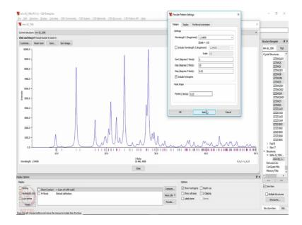
So, a an (Refer Time: 25:29) fw between 0.25 and 0.3 is something what one should use and then simulate the powder pattern. You see here this powder pattern is spread from about 10 degree into theta, to about 45 degree into theta and beyond 50 45 the peaks are very small.
