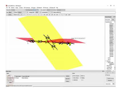
So, now, what we have a 2 planes one plane passing through the terminal carbonic ring terminal aromatic ring and 1 plane passing through the central aromatic ring.
