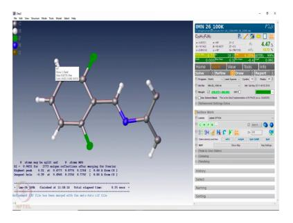
So, that is why we do not try to locate these hydrogens that is we do not assign the residual electron densities as hydrogens rather, we actually calculate those hydrogens from the carbon atoms that is being refined.
