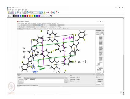
So, this is just the screenshot that I have pasted here. So, that I can write that where is the origin, which is this is the origin, these green once are 2 1 screw and the purple indicates the c glide. Note that if 2 1 screw is one forth shifted along oc and the mirror plane is one forth shifted along ob. So, this is what we learned, when we were trying to draw the space group backgrounds for various space groups in 2 dimension.
