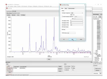
So, generally we simulate up to 50 degree into theta and generally from 30 degree to theta as well. And we see here there is no peak below 10 degree to theta.
