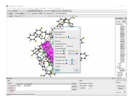
So, here what we can see is that the orange dots that we are seeing here are the inversion centers. So, in case of p 2 1 by c as we have learnt in our class that if you consider the origin at 000, which is the centre of inversion then with respect to that origin the screw axis which is shown here, this green lines are screw axis. Those screw axis are one forth shifted along c, if you look at that from oc, the origin is here the screw axis which is
