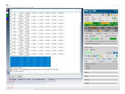
Those hydrogens are now treated separately. They have their corresponding fractional coordinates with some negative as well. And the thermal parameters, the isotropic thermal parameters are all different for different hydrogens and they are refined independently. So, this thermal parameters are not calculated based on the isotropic thermal parameter of the carbon 2 which it is attached rather this hydrogens are refined independently.
