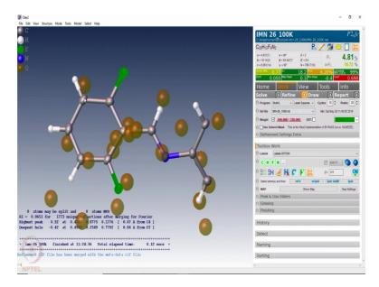
So, after doing H fix 1 has to do a few rounds of refinement to reach convergence on the weighing terms, weighing factors and till you reach the lowest possible r value for particular structure.
