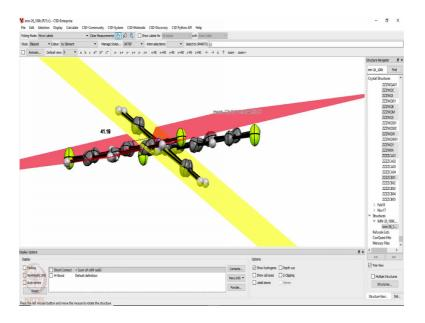
Again you go back and measure angle between the 2 corresponding planes you can move the label to a visible point and see what it is. So, the angle between the 2 planes is found to be 41 bits. So, we can clear again, clear measurement and come back.
