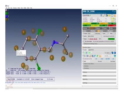
And then we do 10 cycles of refinement, which means it is doing some least squares refinement. That means, what it is doing is from the structure that we have given, it is trying to calculate the structure factors for every hkl and comparing the structure factor generated from the structure that is the calculated structure factor compares with the experimentally observed structure factor amplitudes takes the difference and that difference gives rise to difference in electron density.
