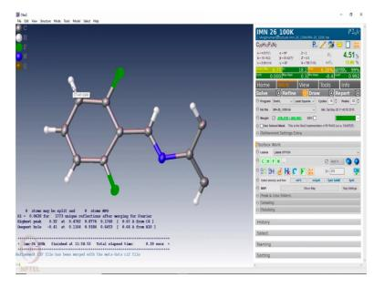
So, here once again we can see that these bond lengths are all same 0.93 angstrom 0.93 and all of them being a single hydrogen connected to sp 3 carbon they have the same bond length 0.93.
