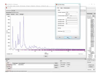
So, now if I change this wavelength to the molybdenum wavelength, which is 0.7109 angstrom or 7.07 angstrom and apply you see the entire pattern which was spread over a large 2 theta value is now squeezed, most of the peaks have merged and it has become more featureless.
