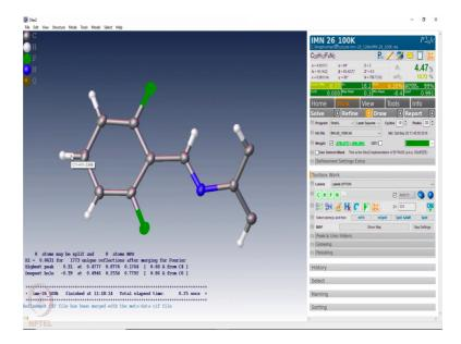
So, here now the distance between the carbon and hydrogen is 9.973, here the distance is 0.948.
