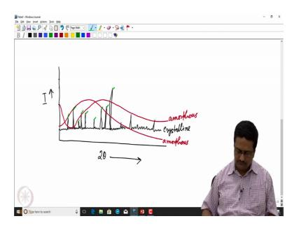
When we shine X-rays on a crystalline substance, we can record its powdered X-ray diffraction pattern. And the pattern would look like the way I am drawing. We plot intensity in the y-axis, and the 2 theta that angle or diffraction in the x-axis. And for a
