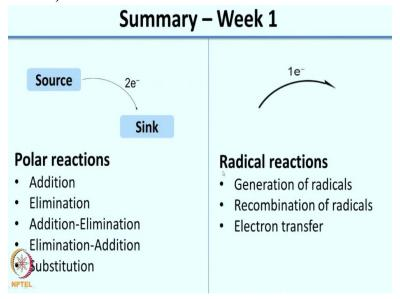
one is the polar reactions and the second is the radical reactions. So, for polar reactions what you do is you use a double headed arrow to show movement of electrons and this double headed arrow indicates movement of 2 electrons. So typically, the arrow originates from the electron source and it goes to the electron sink. So, lot of terms that are used analogous to source is a donor and nucleophile and instead of a sink you would have heard terms like electrophile and acceptor.
