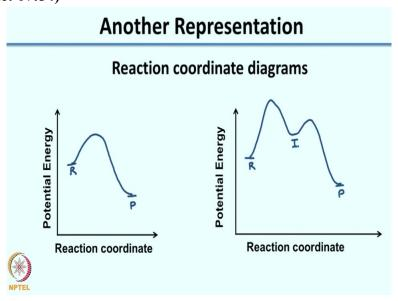
So the reaction co-ordinate diagram typically has your Y-axis which is the potential energy and the X-axis which is called a reaction co-ordinate and what you would see is you would have things which look like this, you would also have reaction co-ordinate diagrams which look like this. So, as you can see both of these diagrams look very different and you can have multiple reaction co-ordinate diagrams.
