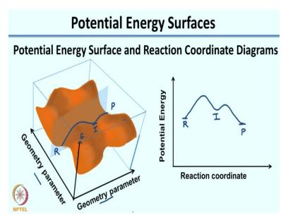
So now so what your potential energy surface is, on this axis you have your energy and on the X and Y axis on Z-axis your energy and on X and Y axis you pick certain parameters you cannot pick all the vibrational modes and these parameters are your geometry parameters analogous through a reaction co-ordinate. So if you look at this complex surface what you would see is this complex surface has multiple hills and multiple valleys. Alright?
