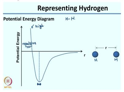
So here I am plotting the potential energy versus the distance between the 2 hydrogen atoms. So when the distance is very very small, so you have these 2 atoms very very close to each other, you have highly repulsive forces. So what happens is the energy is very high. Now as the distance increases, it comes to an optimal distance, this is probably where you have the constructive overlap of the hydrogen atomic orbitals to give you the hydrogen molecule.
