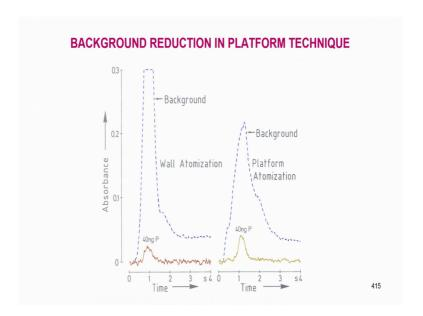
Now this is how the background reduction in platform technique occurs. Look at this the I am trying to determine 40 nano grams of phosphorus. This is the signal peak 40 in this thing, but if I plot the background also you can see the background is So high it crosses c 1.3 absorbance whereas, the sample 40 nano grams of phosphorus is less than 0.01 absorbance here. For 0.01 absorbance a background is 0.3.
