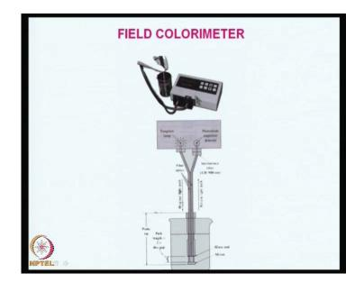
Here, I have shown you a photometric titration in this and here you are adding the reagent and you can take the sample and reference through this and then, put it there and then, measure the absorbance. So, these can be directly connected to the computer to record the absorbance versus volume of the titrant added.
