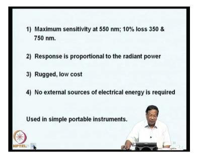
The whole equipment is encased in a glass cell and this photovoltaic cell shows maximum sensitivity at 550 nanometers approximately, 10 percent loss occurs around 350 to 750 nanometers. Therefore, it is basically very rugged instrument and very low
