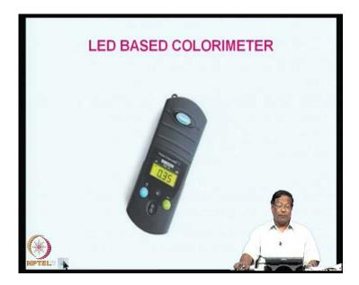
This is a very low led based calorimeter which I was telling that it is something like a filter photometer only, but detected instrument, very low cost and the display here is in terms of concentration. It is a reading 0.035, but it can be any value depending upon the concentration. Now, the slightly higher end equipments are single beam spectrophotometers.
