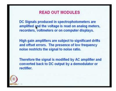
Now, what about the read out modules? How do you read the signal? The DC signals produced in spectrophotometers are usually amplified and the voltage is read on the analog meters or it can be a recorder or a voltmeter or it can be passed on to a computer through RS232 connection and then, computer displays. High gain amplifiers are usually subject to significant drifts and offset errors. Now, the presence of low frequency noise restricts the signal to noise ratio.
