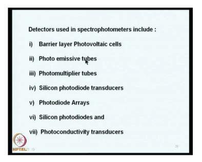
We were discussing detectors used in the spectrophotometers and these includes barrier layer photovoltaic cells, photo emissive tubes, photomultiplier tube, silicon photodiode transducer, photodiode arrays, silicon photodiodes and photoconductivity transducers.
