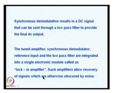
This is very important because unless it is synchronized, you will not get a decent signal at all. So, what you need is a synchronous demodulation and this synchronous demodulation results in a DC signal that can be sent through a low pass filter to provide the final DC output.
