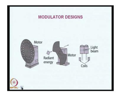
Here, this is a fan. You can see that there are number of holes here and when this fan rotates, light will be passing alternately through this hole and then, it will be blocked again. It will be passed through this hole like that. There are number of possibilities and this is a middle figure is another design or you can do it electronically with a light beam and coils. So, it will just flip-flop here, this side, this side, this side, this side etcetera.
