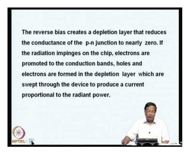
The current will start slowing. Suppose the reverse bias is applied, then the electrons are promoted to the conduction bands and holes and electrons are formed which are swept through the device to produce a current proportional to the radiant power.
