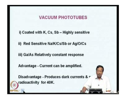
So, the vacuum phototubes cathodes are coated with potassium, cesium, antimony etcetera. These are very highly sensitive for release of the electrons. When the photo, when the light falls on them, red sensitive, sodium, potassium, cesium, antimony are also used or silver and then, oxides cesium etcetera are also used for coating.
