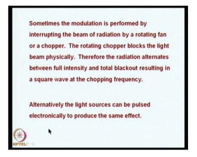
So, this is the type of modulation we normally look for when you use a rotating fan or a chopper. So, alternately they can be done electronically also which we saw that earlier.
