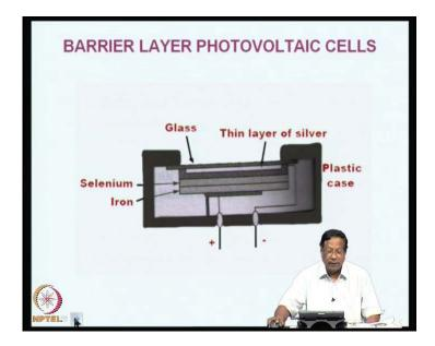
This is a barrier layer photovoltaic cell. Basically it contains two glass plates. One glass plate is here and another is here. It contains a thin layer of silver and a plastic. Everything is coated in plastic and this is a selenium layer which will release electrons when light falls on them and bottom one is iron plate and this iron plate acts as a conductor.
