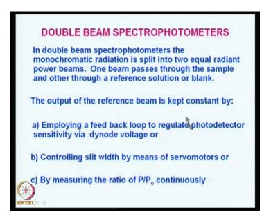
Now, double beam spectrophotometers are always used when the signals are split into two equal radiant power beams. One beam passes through the sample, other through air reference solution or a blank.
