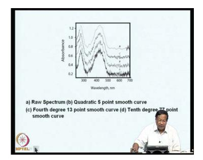
Now, you can see figure A is the raw signal, raw spectrum and figure B, that is this one is a quadratic with 5 point smooth curve. Suppose, we increase it to 4 point fourth degree, then you can see here like this signal is still better and suppose, you increase it to tenth degree 77 point smooth curve, it will give a beautiful signal like this.
