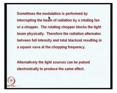
Sometimes the modulation is performed by interrupting the beam of radiation by a rotating fan or a chopper. What you do is the beam or radiation is passing, we just put a fan, so that you can, the beam can be cut physically. You can see the figure here.
