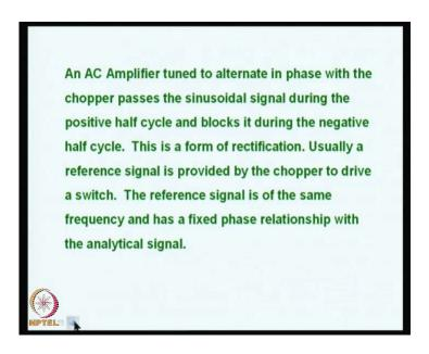
So, an AC amplifier must be tuned to alternate in phase with the chopper that passes the sinusoidal signal during the positive half cycle and blocks it during the negative half cycle. This is a form of rectification basically. Usually a reference signal is provided by the chopper to drive a switch. So, the reference signal is of the, should also be of the same frequency and has a fixed phase relationship with the analytical signal.
